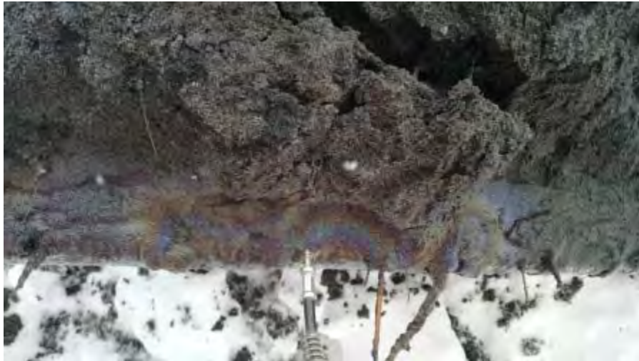
March 3, 2015 - Excavated soil with sheen in excavation bucket.
