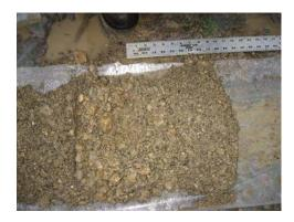
32.5 to 38.0' Sand, medium to Pebbles, coarse; sub-round to sub-angular; trace silt; poorly sorted; wet; grayish brown (10YR5/2). NOTE: sedimentary, igneous and metamorphic particles.
