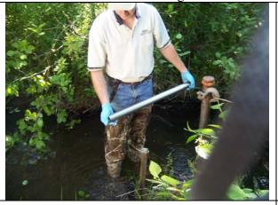
Next a composite Sediment sample was collected. The samples were only collected to a depth of 6-inches. Any sediment that was collected in the sampling tube at a depth greater than 6-inches was discarded.
