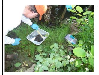
Once the proper amount of sediment is collected. The composite sample is mixed to a homogenous sample.
