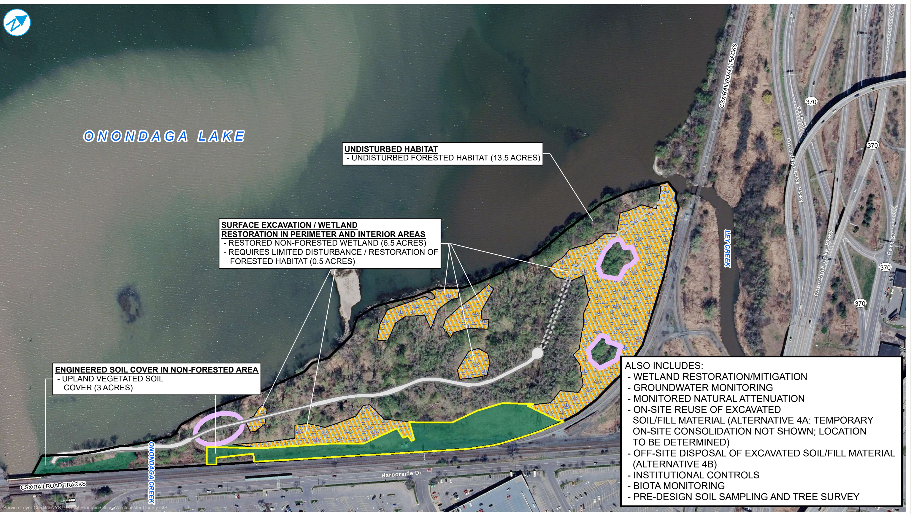
SYW-12 ALTERNATIVE 3A/B SURFACE EXCAVATION AND ENGINEERED COVER / RESTORATION ON PERIMETER AND INTERIOR AREAS (10 ACRES), BIOTA MONITORING, AND MNA, WITH LIMITED TREE REMOVAL
