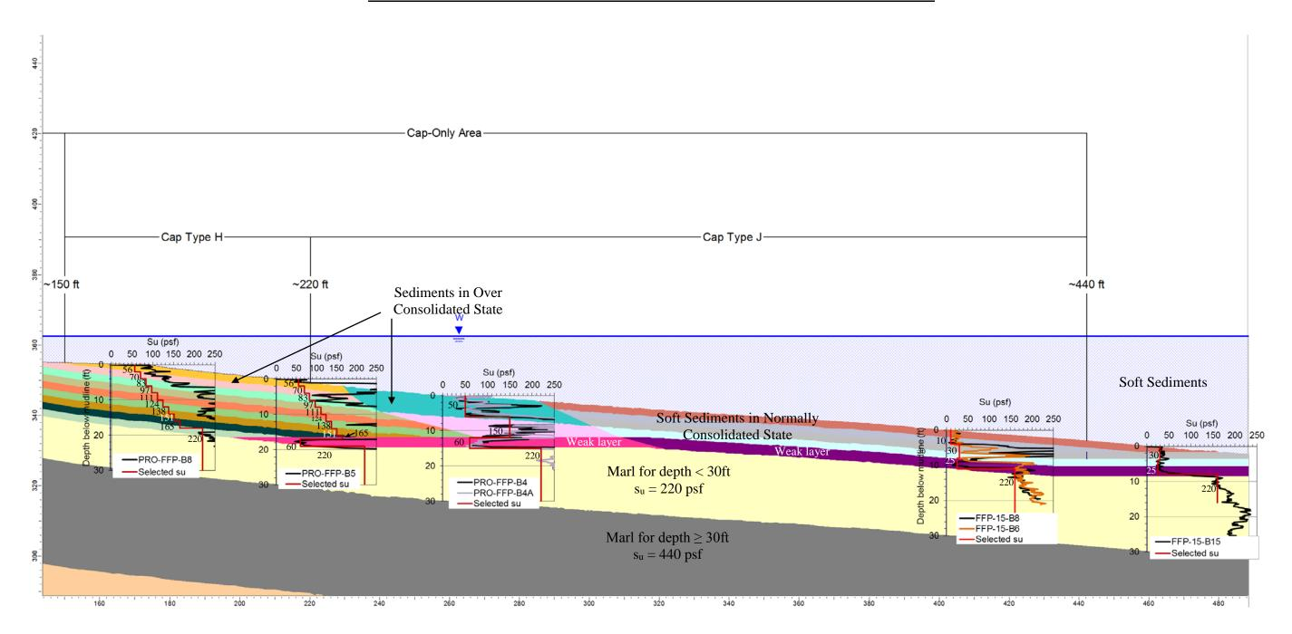
Figure 5. Subsurface stratigraphy and shear strength (s<sub>u</sub>) profiles from the FFPs collected near Cross Section C
