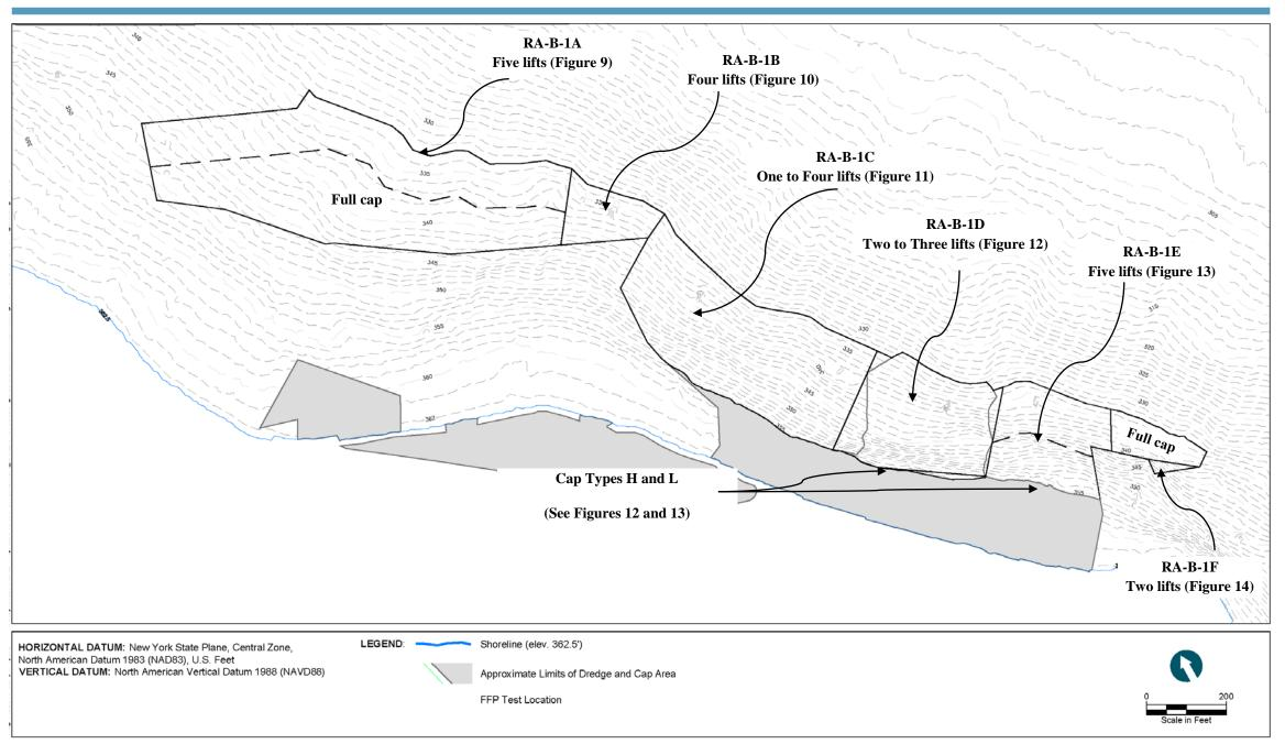
Figure 15. Recommended cap placement in modified protective cap area RA-B-1
