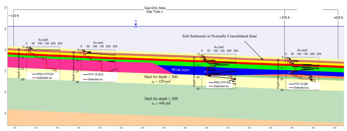
Figure 3. Subsurface stratigraphy and shear strength (s<sub>u</sub>) profiles from the FFPs collected near Cross Section A. The values on the profiles show the selected shear strengths in psf.
