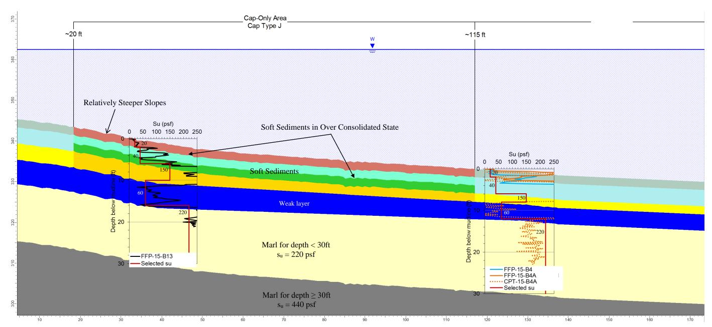
Figure 8. Subsurface stratigraphy and shear strength (s<sub>u</sub>) profiles from the FFPs collected near Cross Section F
