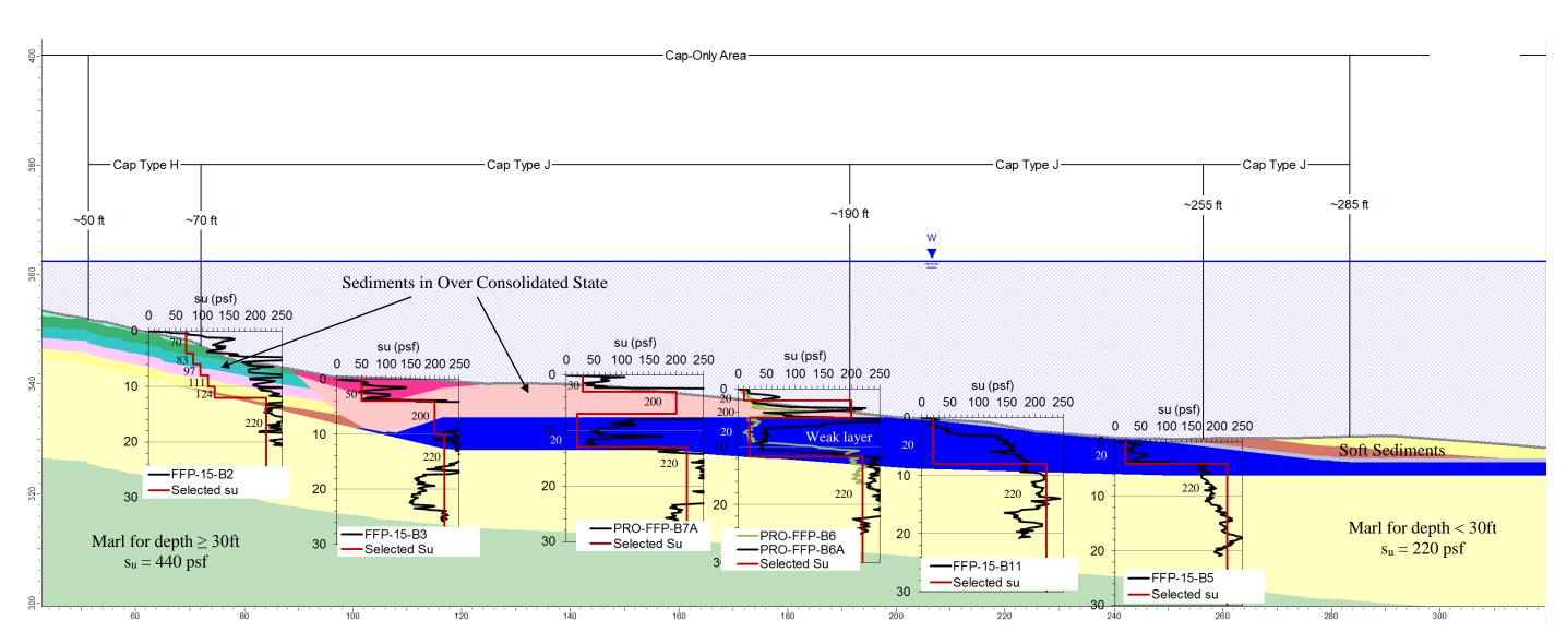
Figure 6. Subsurface stratigraphy and shear strength (su) profiles from the FFPs collected near Cross Section D
