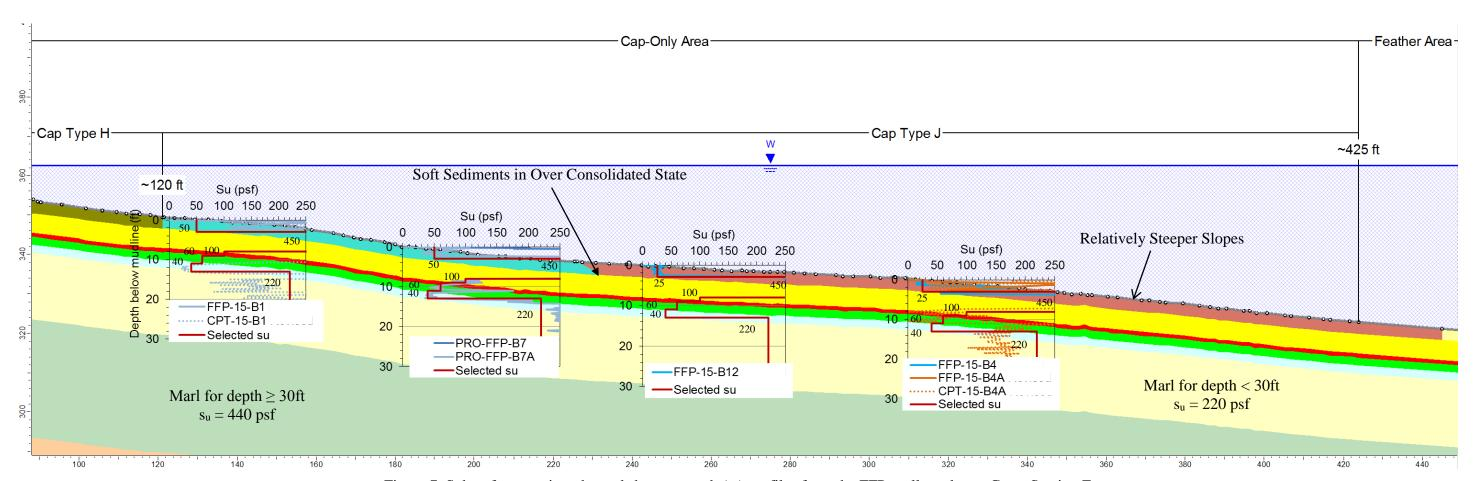
Figure 7. Subsurface stratigraphy and shear strength (su) profiles from the FFPs collected near Cross Section E
