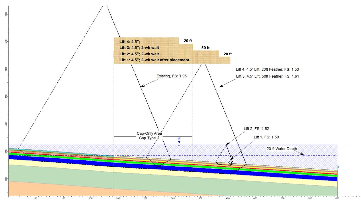
Figure 10. Calculated factors of safety and critical slip surfaces in Cross Section B for various cap placement conditions
