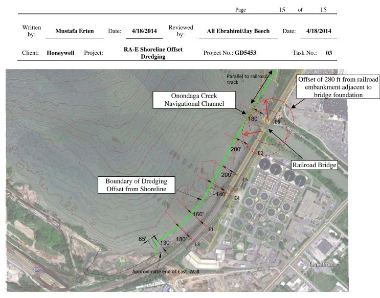
Figure 10. Minimum Required Dredge Offset Distance and Recommended Boundary of No-Dredging Area
