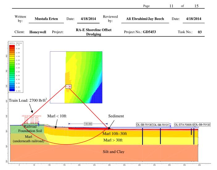
Figure 6. Geometry and Slope Stability Analysis Results of Cross Section E3 (with Offset Distance of 130 ft from the Shoreline)
