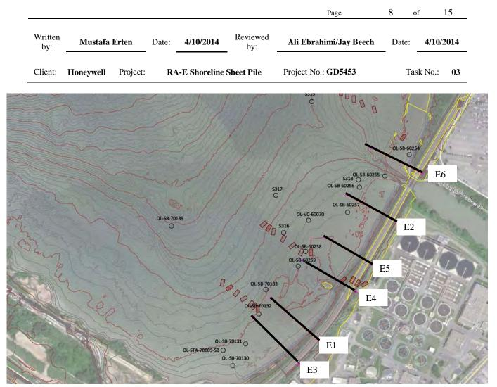
Figure 1. Locations of Selected Six Cross Sections and Available Soil Borings
