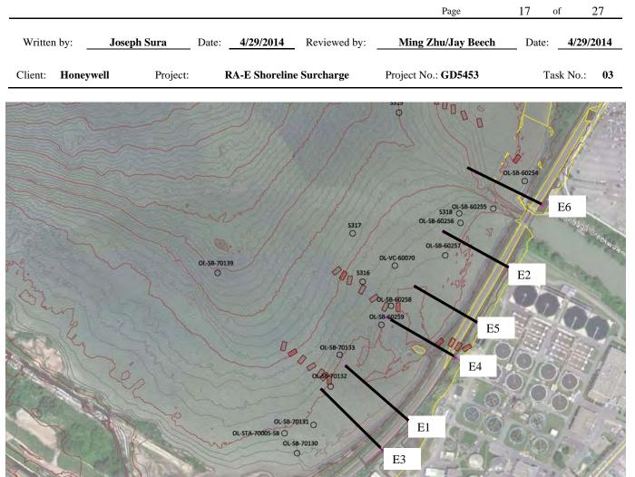
Figure 2. Locations of Selected Six Cross Sections for Stability and Available Soil Borings
