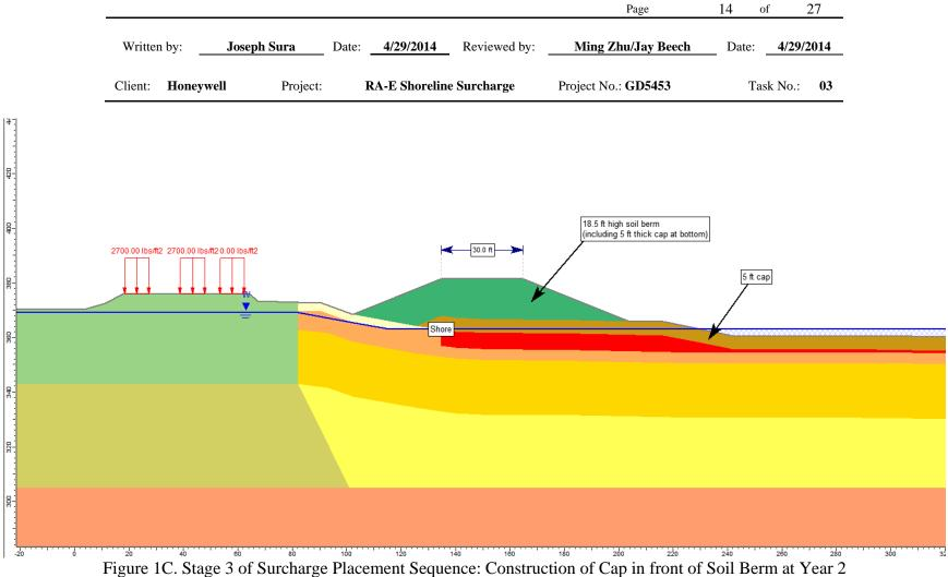
Note: Settlement that will occur under the soil berm is not illustrated in the figure.
