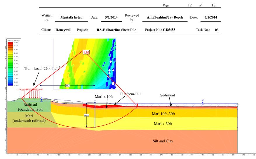
Figure 5. Geometry and Slope Stability Analysis Results of Cross Section E4 where sheetpile is 30 ft away from the shoreline
