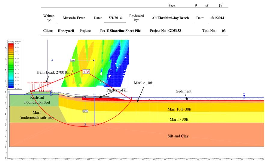
Figure 2. Geometry and Slope Stability Analysis Results of Cross Section E1 where sheetpile is 30 ft away from the shoreline
