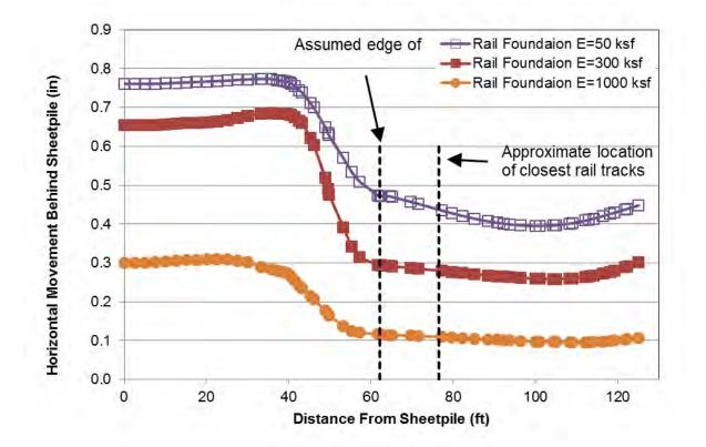
Figure 10. Sensitivity of Calculated Horizontal Deformation to Modulus of Railroad Foundation at Cross Section E5 where sheetpile is located 30 ft away from the shoreline (Railroad Foundation Soil Modulus, E = 50, 300, and 1000 ksf)
