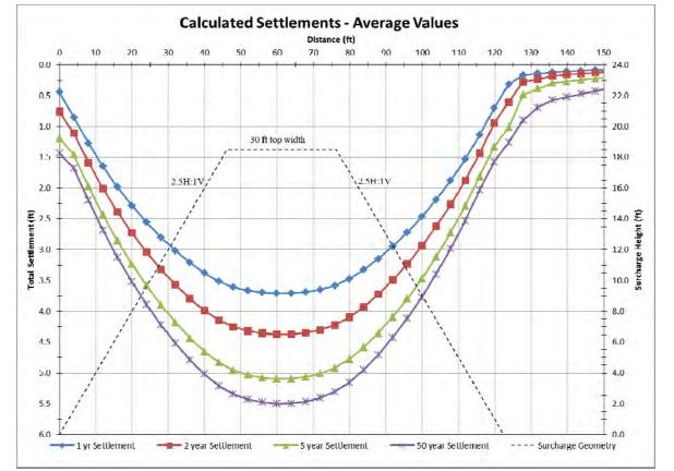
Figure 11. Calculated Primary Consolidation Settlement at Different Times using Average Consolidation Parameters: 18.5- ft Surcharge Note: The distance is measured from the toe of the surcharge inside the lake (i.e., 0 ft indicates the toe of the surcharge in the lake and 122.5 ft indicates the toe of the surcharge on land).
