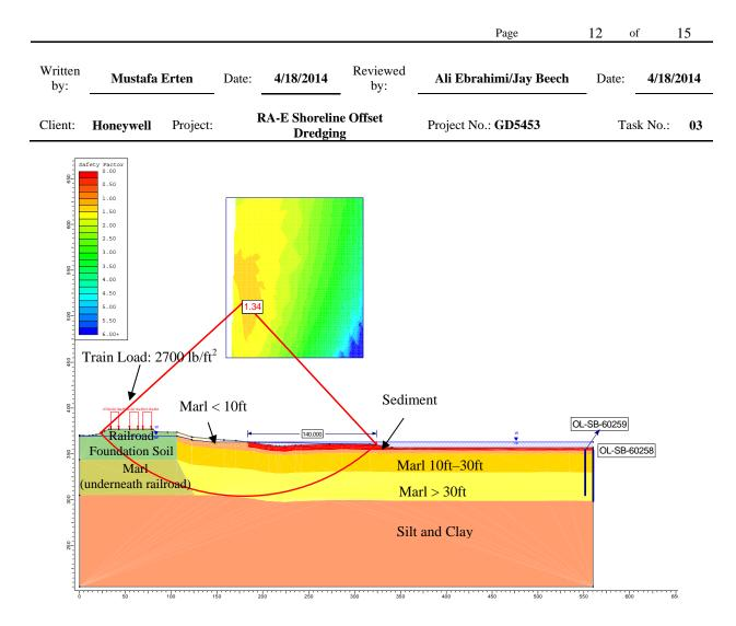
Figure 7. Geometry and Slope Stability Analysis Results of Cross Section E4 (with Offset Distance of 140 ft from the Shoreline)
