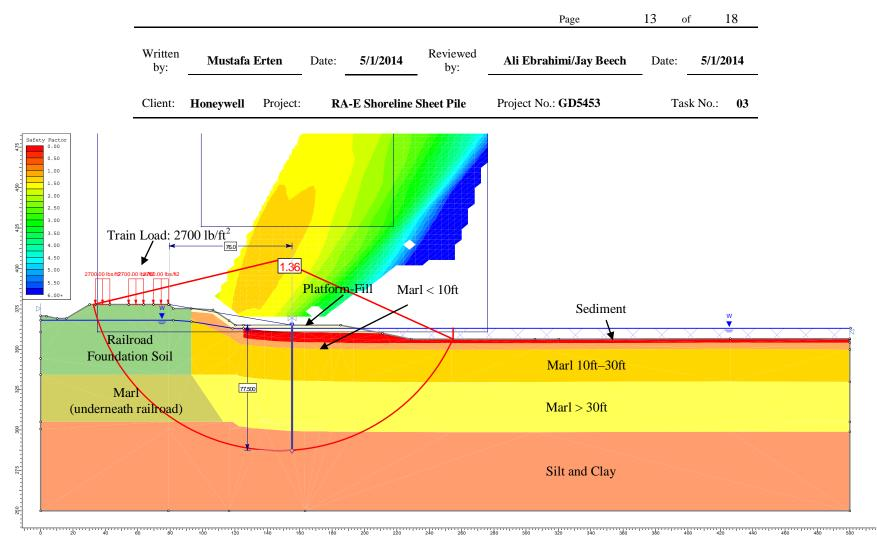
Figure 6. Geometry and Slope Stability Analysis Results of Cross Section E5 where sheetpile is 30 ft away from the shoreline
