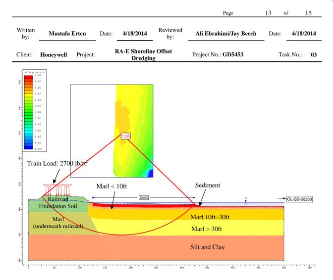
Figure 8. Geometry and Slope Stability Analysis Results of Cross Section E5 (with Offset Distance of 200 ft from the Shoreline)
