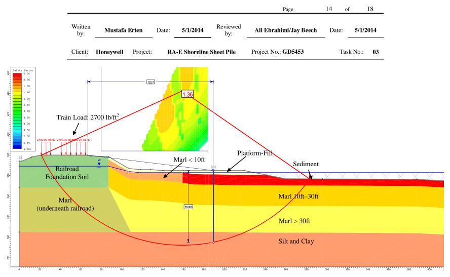
Figure 7. Geometry and Slope Stability Analysis Results of Cross Section E6 where sheetpile is 30 ft away from the shoreline
