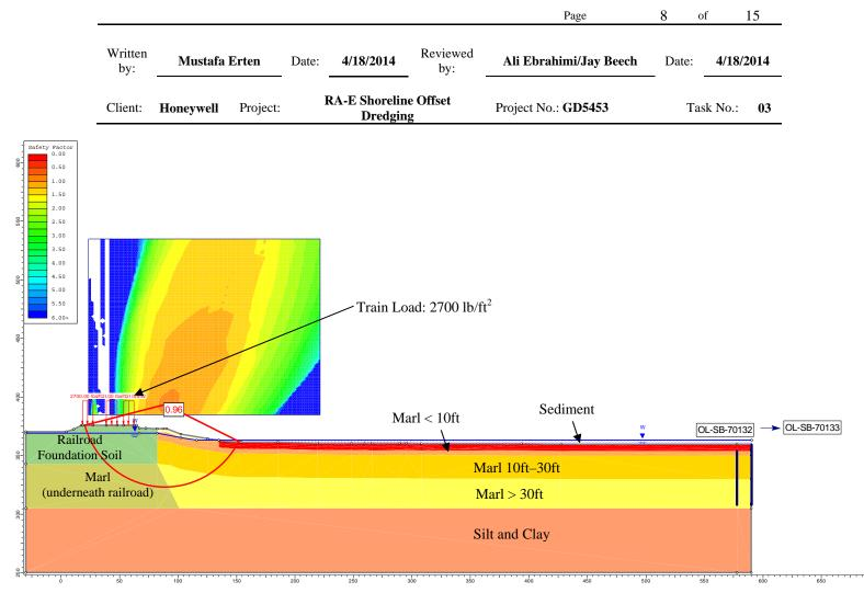
Figure 3. Slope Stability Analysis Results of Cross Section E1 for the Existing Condition
