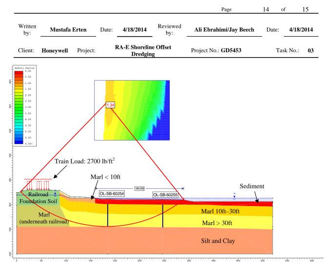
Figure 9. Geometry and Slope Stability Analysis Results of Cross Section E6 (with Offset Distance of 180 ft from the Shoreline)
