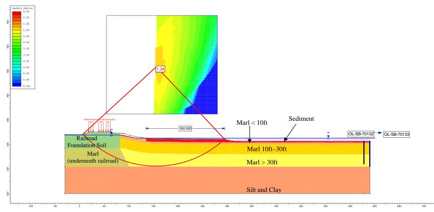
Figure 4. Geometry and Slope Stability Analysis Results of Cross Section E1 (with Offset Distance of 160 ft from the Shoreline)
