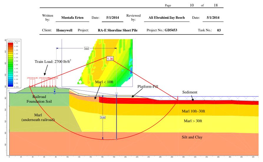
Figure 3. Geometry and Slope Stability Analysis Results of Cross Section E2 where sheetpile is 30 ft away from the shoreline
