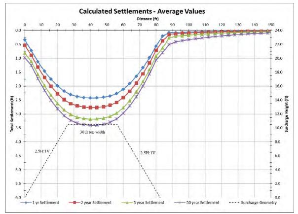
Figure 12. Calculated Primary Consolidation Settlement at Different Times using Average Consolidation Parameters: 10.5- ft Surcharge Note: The distance is measured from the toe of the surcharge inside the lake (i.e., 0 ft indicates the toe of the surcharge in the lake and 82.5 ft indicates the toe of the surcharge on land).
