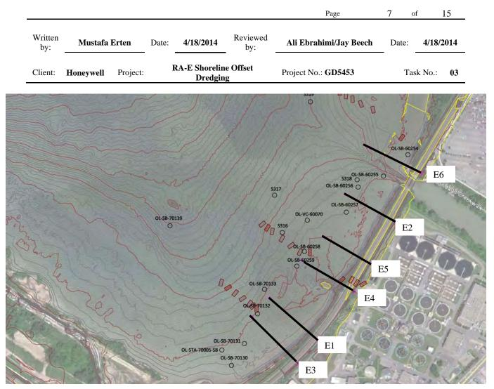
Figure 2. Locations of Selected Six Cross Sections and Available Soil Borings
