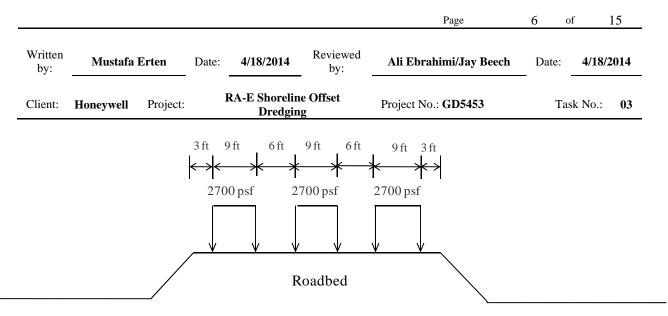
Figure 1. Configuration of Railroad Loading
