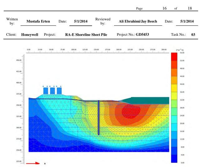
Figure 9. Calculated Deformation Contours after Dredging in front of Sheetpile at Cross Section E5 (Railroad Foundation Soil Modulus, E = 1000 ksf)
