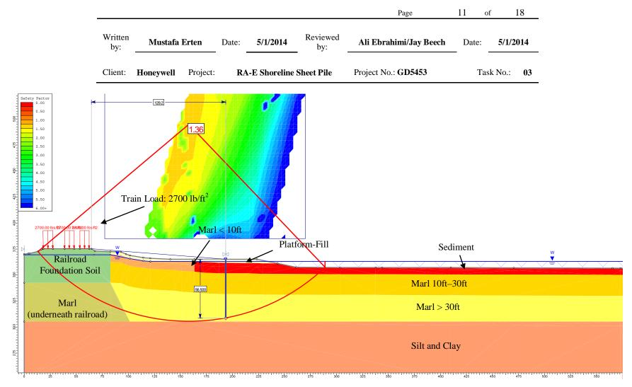
Figure 4. Geometry and Slope Stability Analysis Results of Cross Section E3 where sheetpile is 30 ft away from the shoreline
