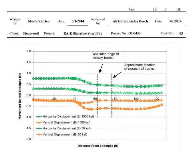
Figure 11. Calculated Vertical and Horizontal Deformation Profiles at Cross Section E5 where sheetpile is located 30 ft away from the shoreline (Railroad Foundation Soil Modulus, E = 50 and 1000 ksf)
