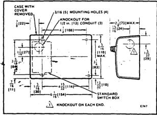
FIG. 1-T631 INSTALLATION DIMENSIONS. [mm SHOWN IN BRACKETS].
