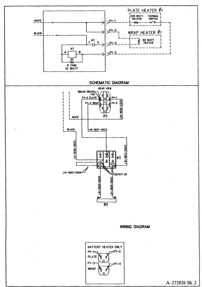
Figure 2a. Battery Heater Kit Electrical Connections (Kit PA-258885)
