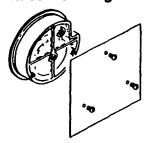
Locate mounting holes, 120° apart on a 4-1/8" dia. circle. Use No. 6-32 machine screws of appropriate length.
