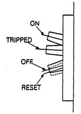
Figure 3. Handle positions for ON, TRIP, and OFF.
