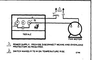
FIG. 3—T631A OR C HOOKUP FOR CONTROLLING FAN.
