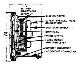
Series 1910 pressure switch. All pressure and electrical connections and set point adjustments are on one side for easy installation.
