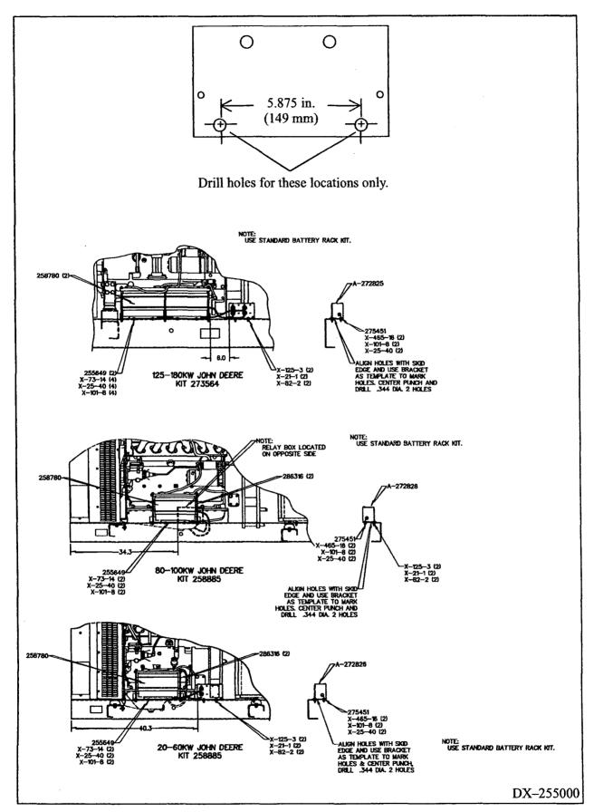
Figure 1a. Installing Battery Heater
