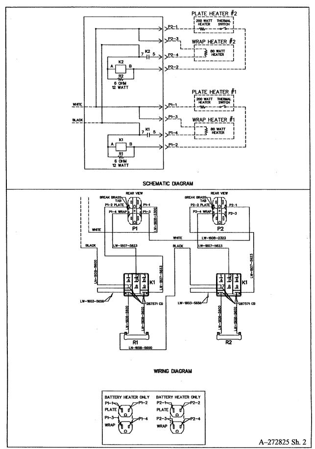
Figure 2b. Battery Heater Kit Electrical Connections (Kit PA-272825)
