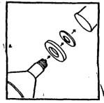
8) Place a fiber washer into each of the light sockels. Then place the rubber gaskets around each socket and a floodlight into A each of the light sockets. DO NOT EXCEED THE 150 WATT MAXIMUM PAR BULB RATING PER SOCKET. Your installation is now complete!
