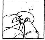
7) Carefully pack all the wires into the junction box. Mount the motion detector over the junction box with the mounting bolt proteging through the center hole in the the mounting bolt until light.
