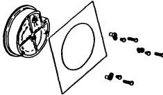
Provide a 4% dia. opening in panel. Insert gage and secure in place with No. 6-32 machine screws of appropriate length, with adaptors, Part No. 360c, firmly secured in place. To mount gage on 14"-2" pipe, order optional A-610 pipe mounting kit.
