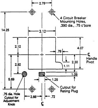
Figure 1. Mounting hole and escutcheon cutout pattern.
