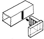
Fig. 1 - Installation drawing of flanged heater.
