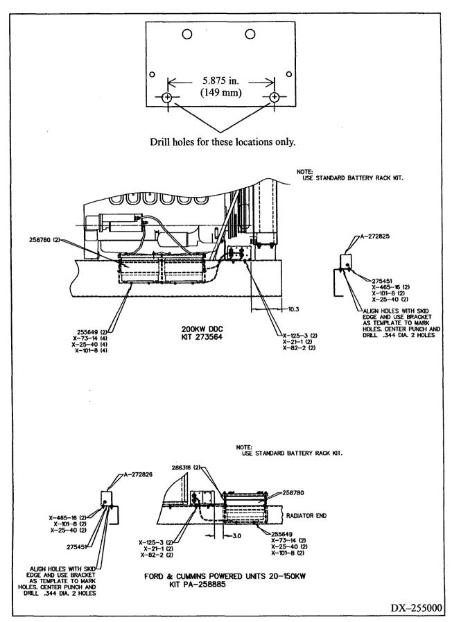
Figure 1b. Installing Battery Heater
