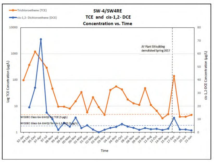
Figure 6-3 Concentration vs. Time, TCE and cis-1,2-DCE in Well SW-4/4RE, Former AFP 59
