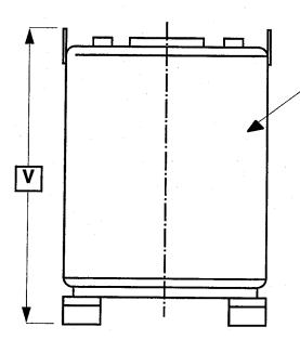
45.5"DIA, D.O.T.RATED, WETTED PARTS EPOXY LINED MILD STEEL. (11 PSI DESIGN PRESS)
