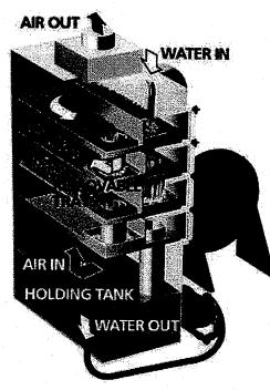
As contaminated groundwater enters through the top of the air stripper, millions of air bubbles are forced by the blower pressure up through the perforated trays, vigorously aerating the water to a froth and removing volatile contaminants (VOC) as gravity pulls the water down through each tray.
