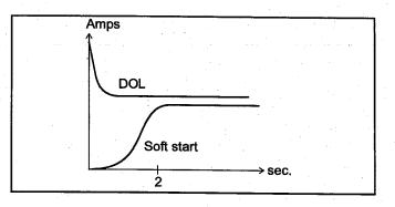
The soft-start will reduce your chance of water hammer, minimizes the risk of wear and prevent overloading of your circuit during start-up.
