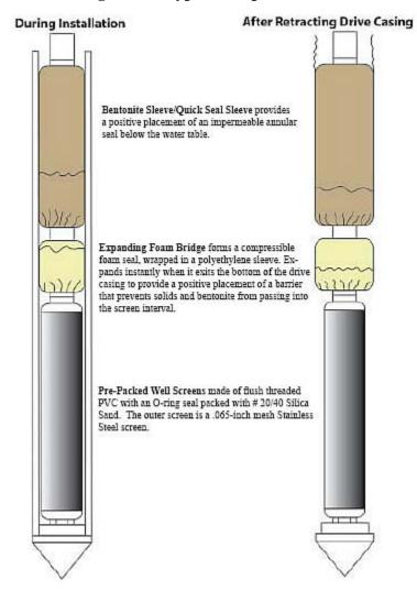
Figure 5-3 Typical Prepacked Well
