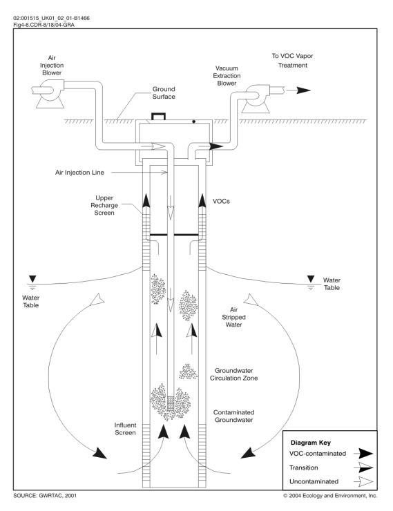
Figure 4-6 Typical NoVOCs Well Construction
