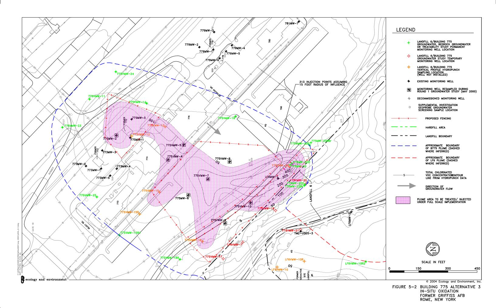
offset horizontally as well as vertically from adjacent wells to facilitate complete distribution of the oxidant throughout the aquifer. For costing purposes, average well depths were assumed for well installations. The injection well configuration and target intervals will be refined during the design. Field parameters such as ORP, conductivity, and water levels will be collected during the injection activities to assess oxidant distribution in the subsurface.
