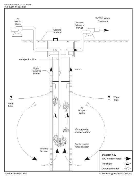
Figure 6-5 Typical NoVOCs Well Construction
