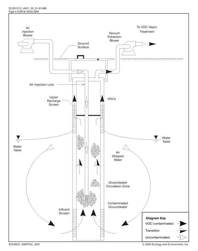
Figure 5-4 Typical NoVOCs Well Construction
