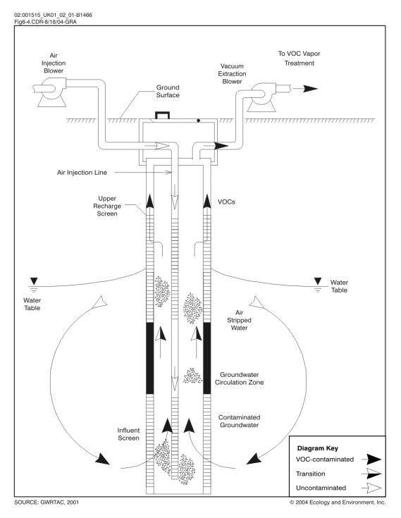
Figure 6-4 Typical Density-Driven Convection (DDC) Well Construction
