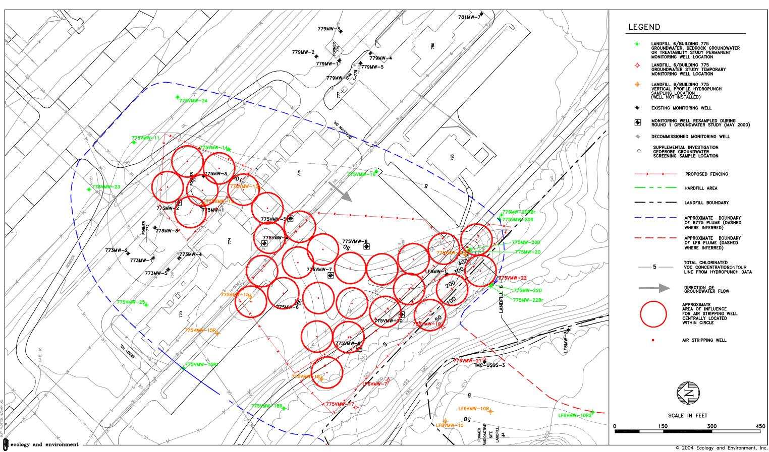
FIGURE 5-6 BUILDING 775 ALTERNATIVE 4 IN-WELL AIR STRIPPING FORMER GRIFFISS AFB ROME, NEW YORK
