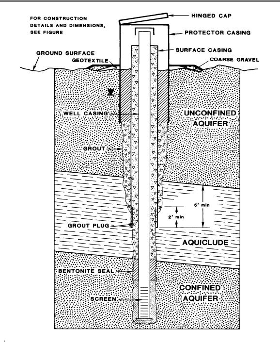
Figure 19.3. Typical well installation, confined aquifer.
