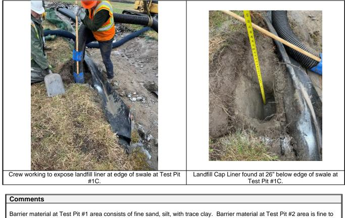
Barrier material at lest Pit #1 area consists of fine sand, slit, with trace clay. Barrier material at lest Pit #2 area is fir medium sand with trace silt.
