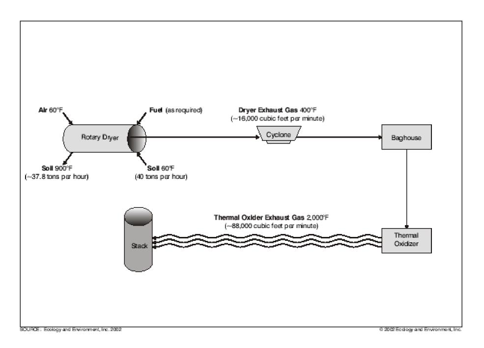
Figure 11 High-temperature Thermal Mass and Energy Balance Luzeme Road Site
