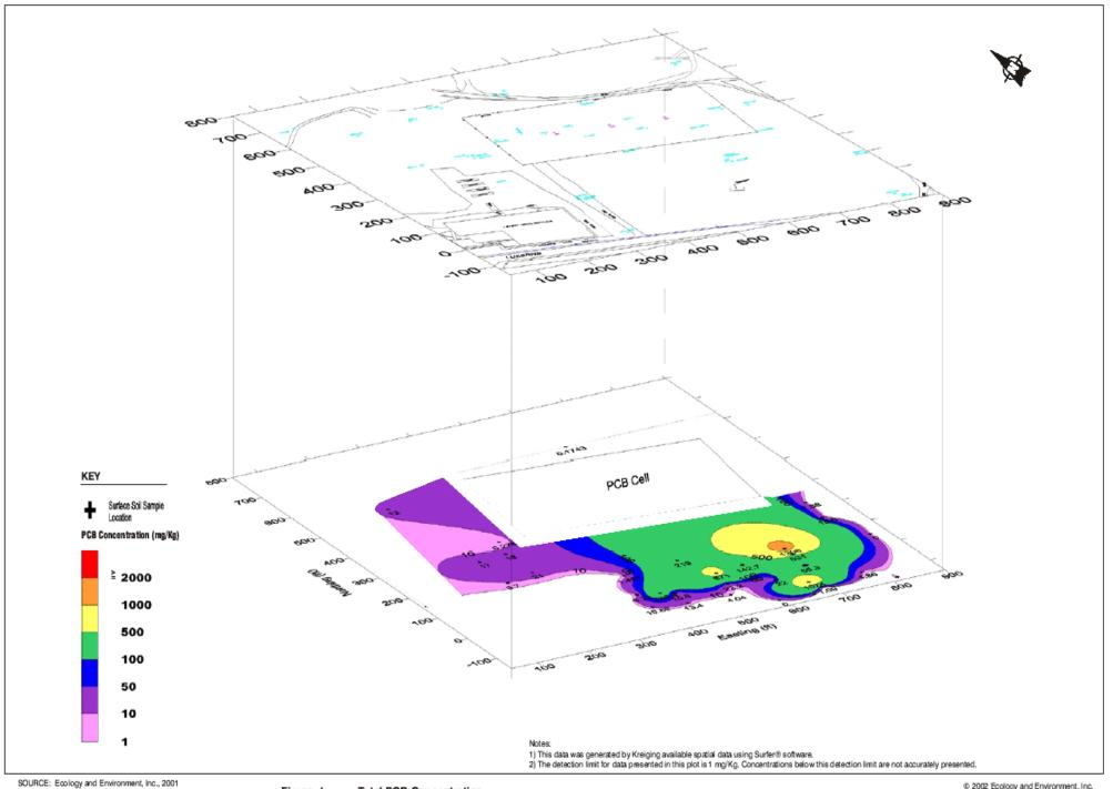
Figure 4 **Total PCB Concentration** Distribution in On-site Surface Soils Luzerne Road Landfill Site Queensbury, New York
