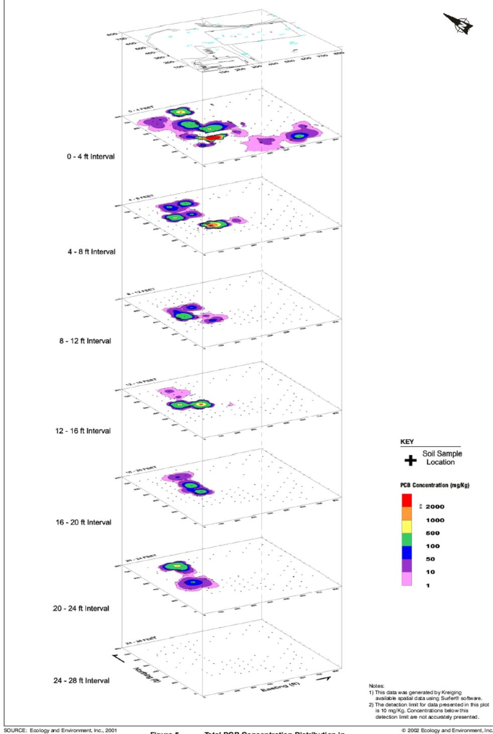
Total PCB Concentration Distribution in Figure 5 On-site Subsurface Soils Luzeme Road Landfill Site Queensbury, New York
