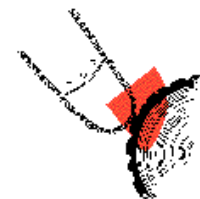
Improper starting of bore
