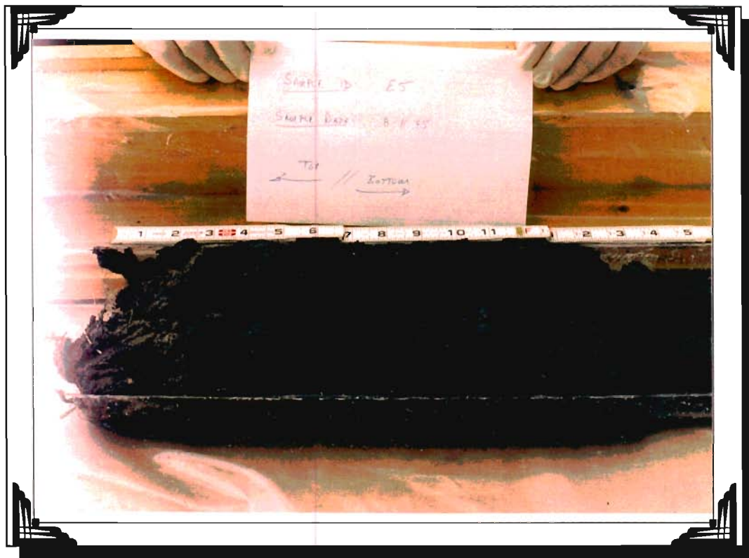
Photo 11: Core sample E-5 illustrating sludge material with interlayering of wood chips.
