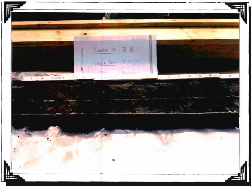
Photo 6: Core sample B-8 illustrating boundary between sludge and sand layers.
