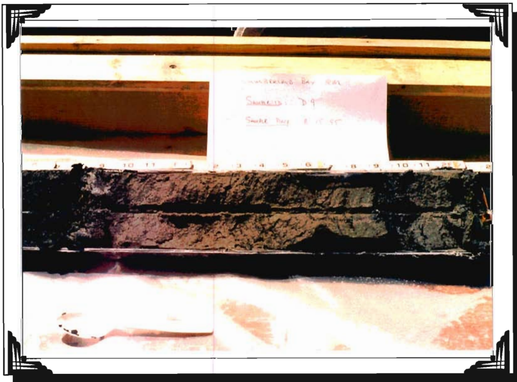
Photo 10: Core sample D-9 depicting the boundary between sludge and sand at the 10-inch interval. Note wood chip layer at base of sample.
