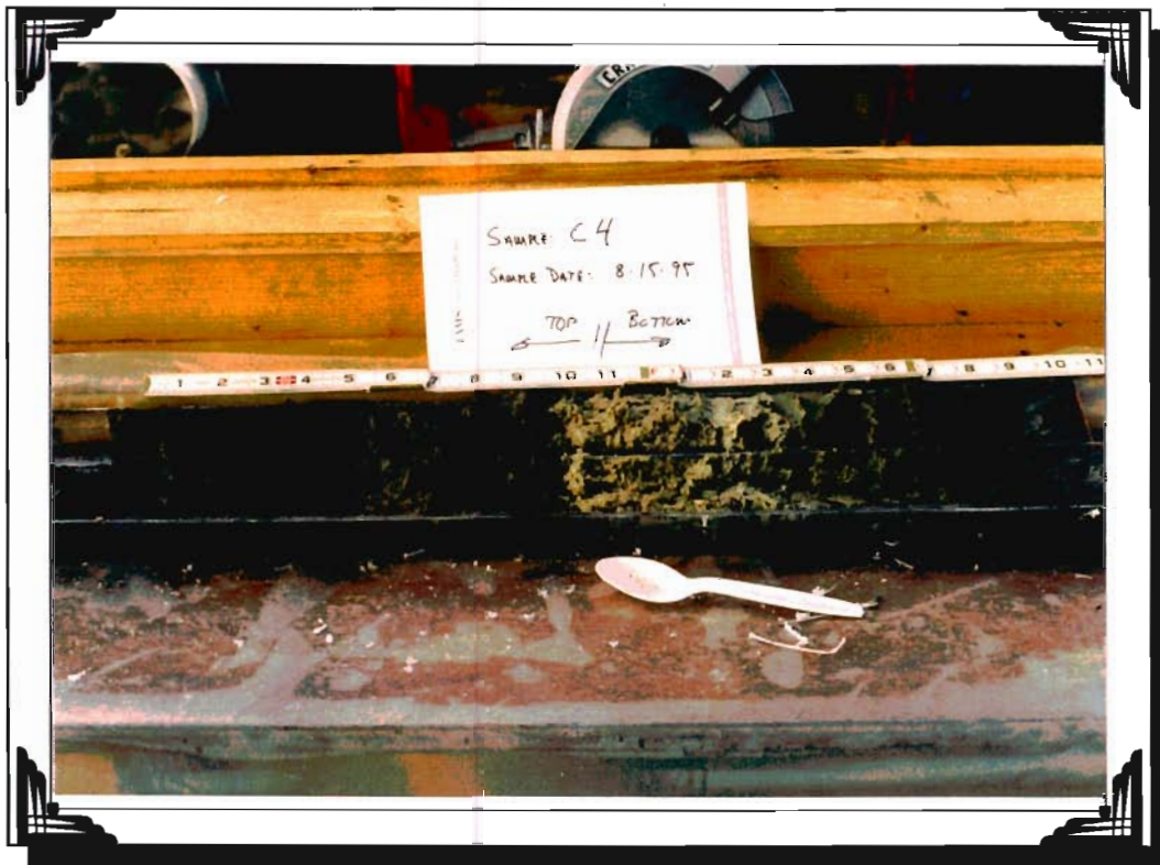
Photo 7: Core sample C-4 illustrating dark sludge layer (top of core) and white paper pulp sludge near center of core.
