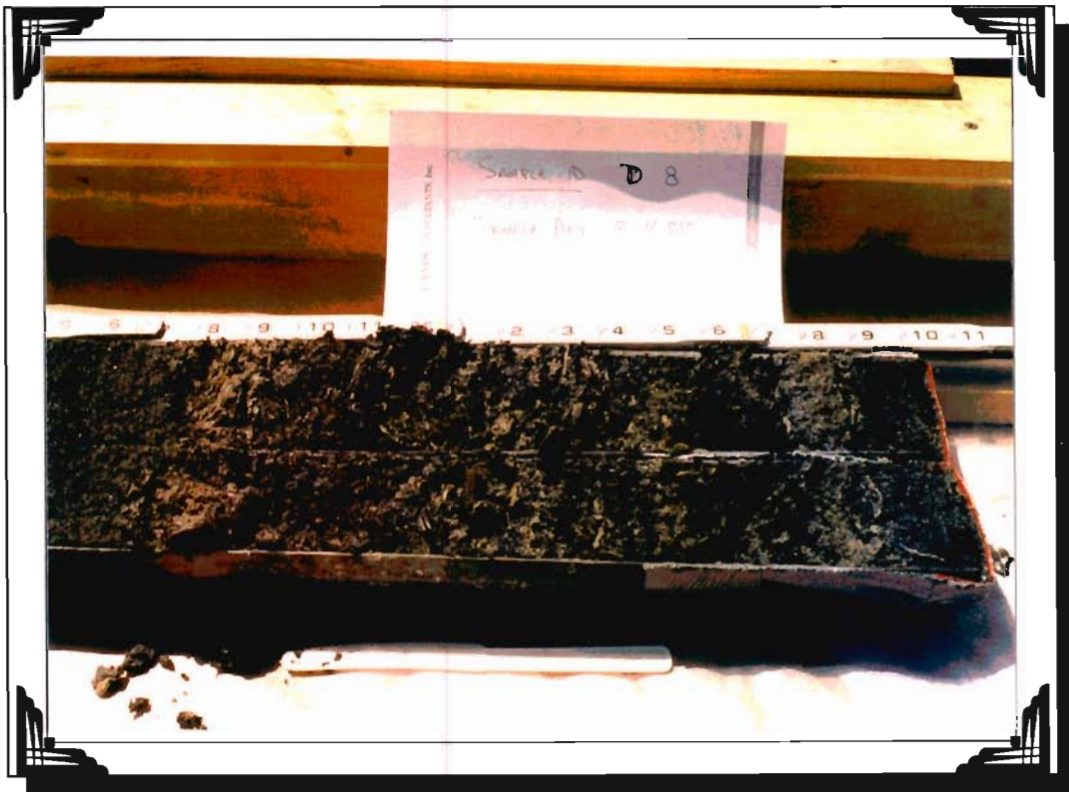
Photo 9: Core sample D-8 illustrating sludge with extensive wood chip material.
