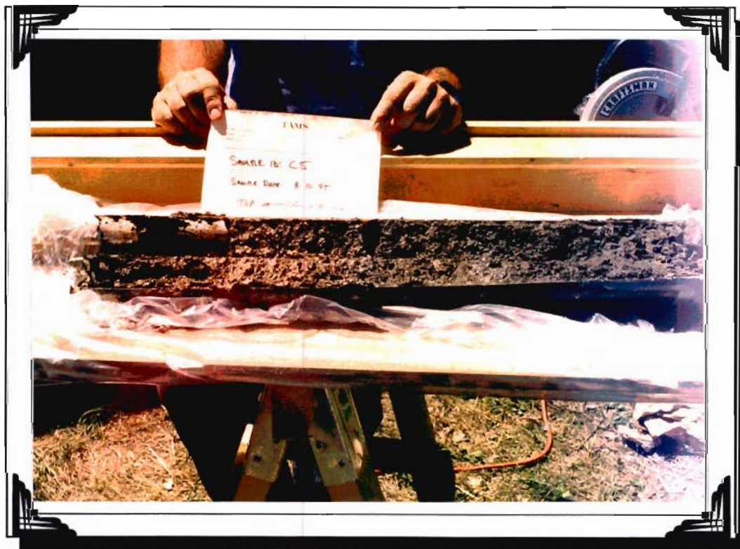
Photo 8: Core sample C-5 illustrating wet, organic sludge.
