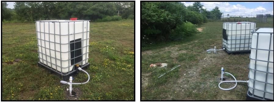
Site 6 – Injection Setup and Injection into IP 4.
