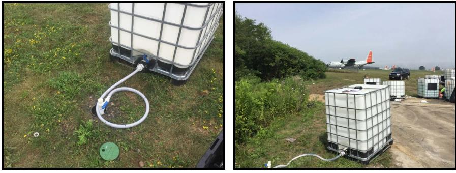
Site 6 – Injection Setup and Injection into IP 5.
