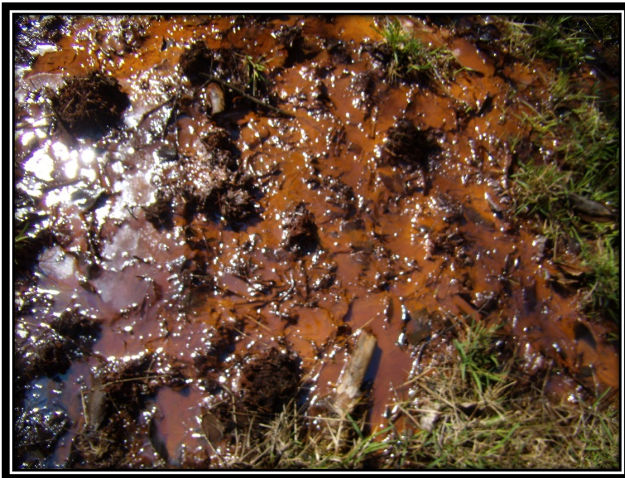
Photos 4 and 5: Leachate impacted surface water area (LISWA) #1 located on the western toe of the landfill indicative of landfill impacted groundwater in the form of orange iron floc deposits and iron bacteria film.
