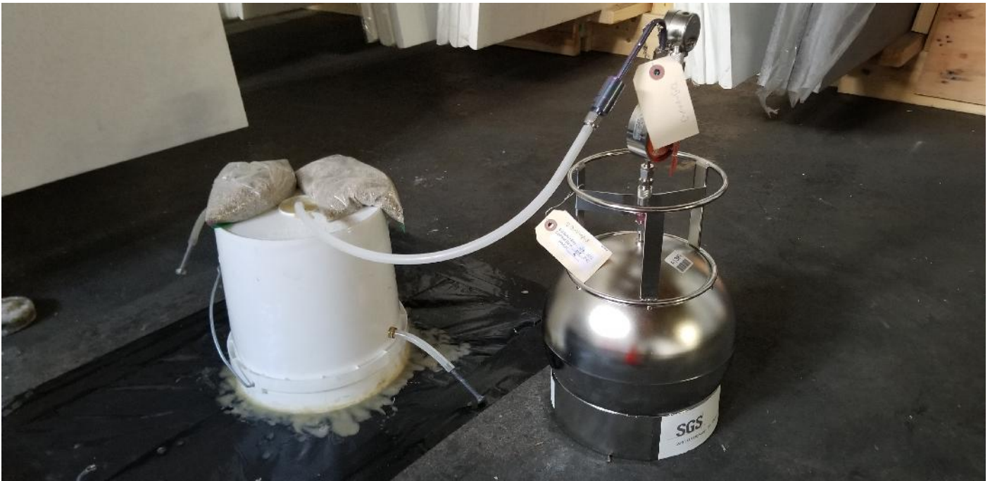
Picture 9: DB-VMP-3 sampling location with tracer gas “flux” chamber
