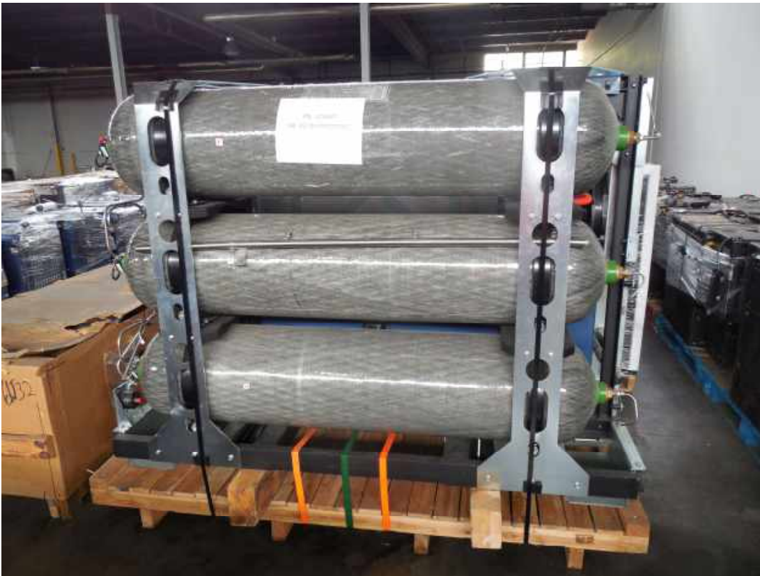
Picture 6: Hydrogen Tanks (PID: 885 ppbv)
