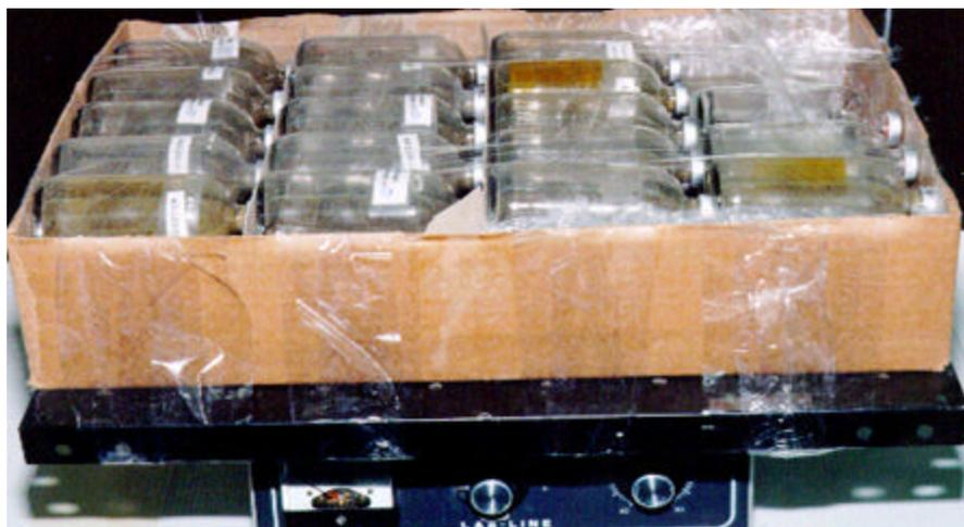
**Figure 4: Soil Slurry Mixing**
