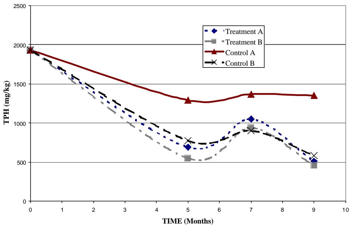
**Figure7: TPH Results from Soil-column Evaluation**
