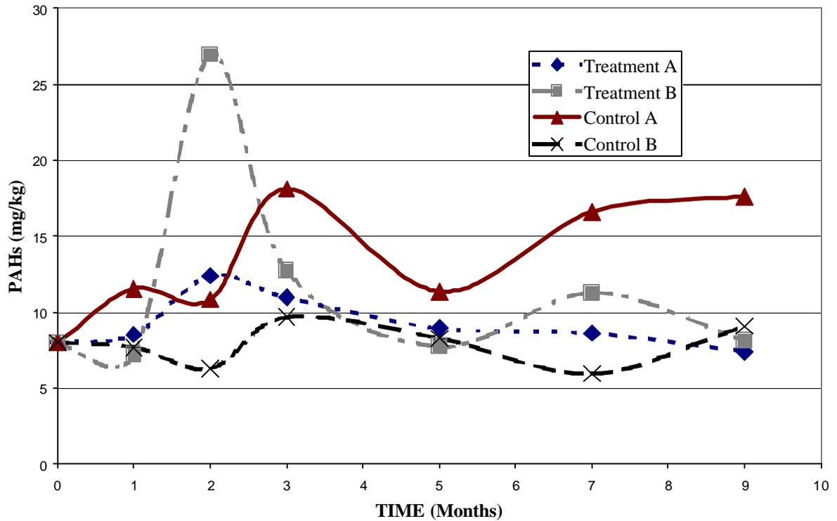
Figure 9: PAH Results from Soil-column Evaluation
