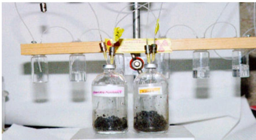
**Figure 2:  $^{14}\text{CO}_2$  Sparging-train System**
