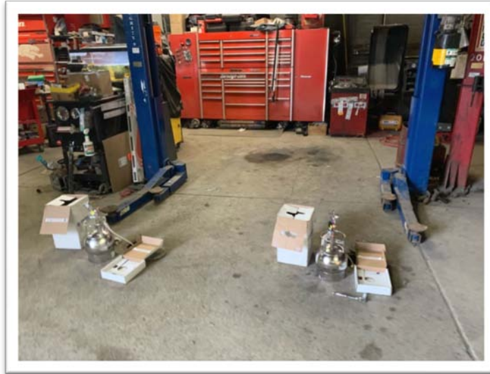
1. Air Sampling at the SVE Points by Using Suma-Canister
