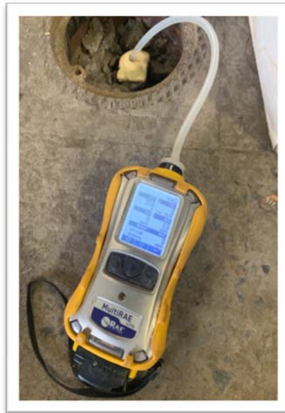
3. A Typical PID Reading by Using MultiRAE
