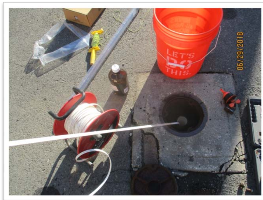
10. Groundwater Level Measurement Using by Solinst Interface Meter
