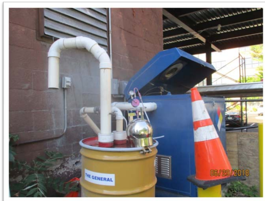
2. Air Sampling at the Discharge of the Carbon Vessel by Using Suma-Canister
