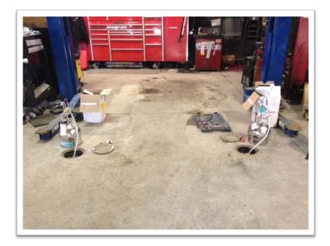
1. Air Sampling at the SVE Points by Using Suma-Canister
