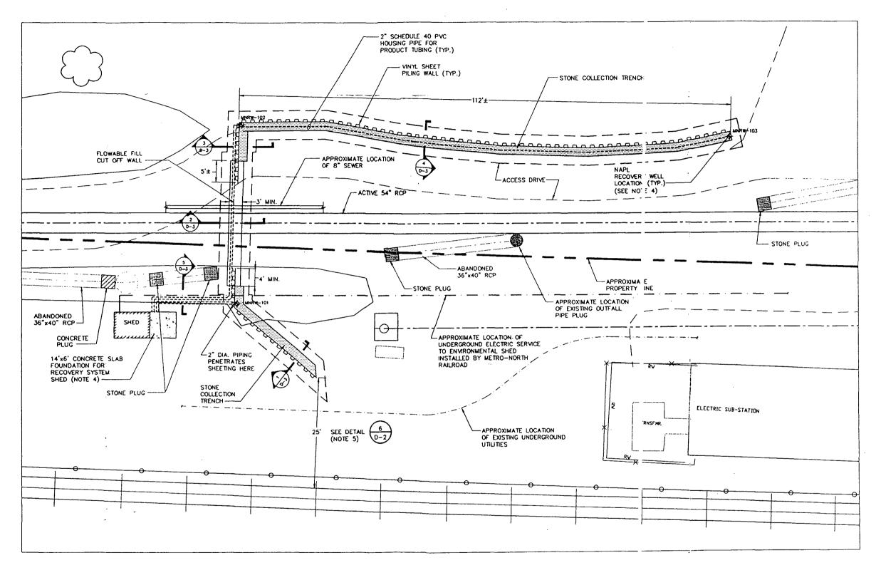
SHEET PILING WALL - STONE COLLECTION TRENCH PLAN VIEW
