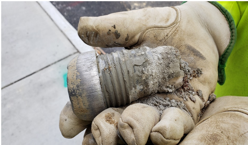
CORE SHOE SAMPLE – PROBE REFUSAL
