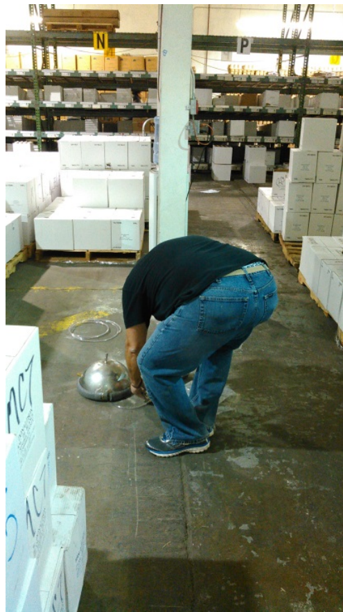
Photo No. 8: Conducting helium testing at sample port LCS-1 in Rental Space A2.
