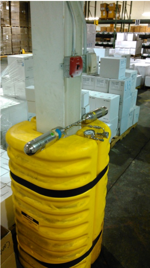
Photo No. 9: Indoor Air sample canisters IA-A2 and IA-A2 duplicate in Rental Space A2.
