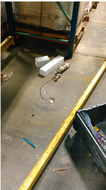
Photo No. 3: Collecting sub-slab vapor sample from port CHA-V10.
