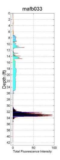
Soil Logging with Laser Induced Fluorescence
