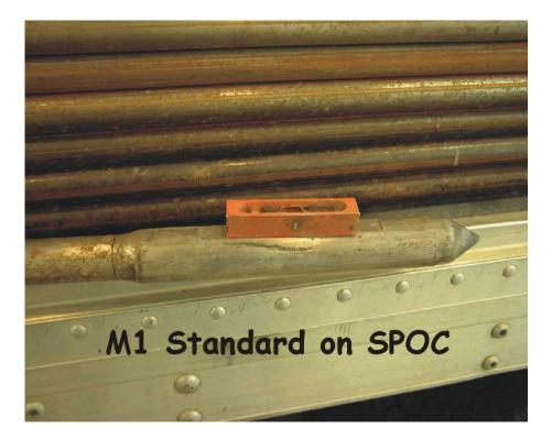
After acquiring the reference waveform, the software will ask if you want to zero the DCAM. Remove the M1 and place the probe under the hammer. Push the probe into the ground until the window is at ground level, this will be zero feet or ground surface. Now start the logging software by confirming that the window is at zero and data acquisition can begin. DCAM should beep, indicating that the push can begin.
