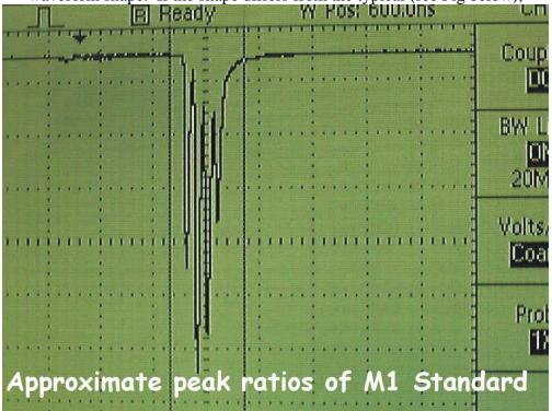
then some parameter of the system in not adjusted properly. If the parabolic mirror in the SPOC is out of adjustment, too much laser light is reflected back into the signal fiber and causes a signal addition to the baseline. See the maintenance section for adjustment of the parabolic mirror.
