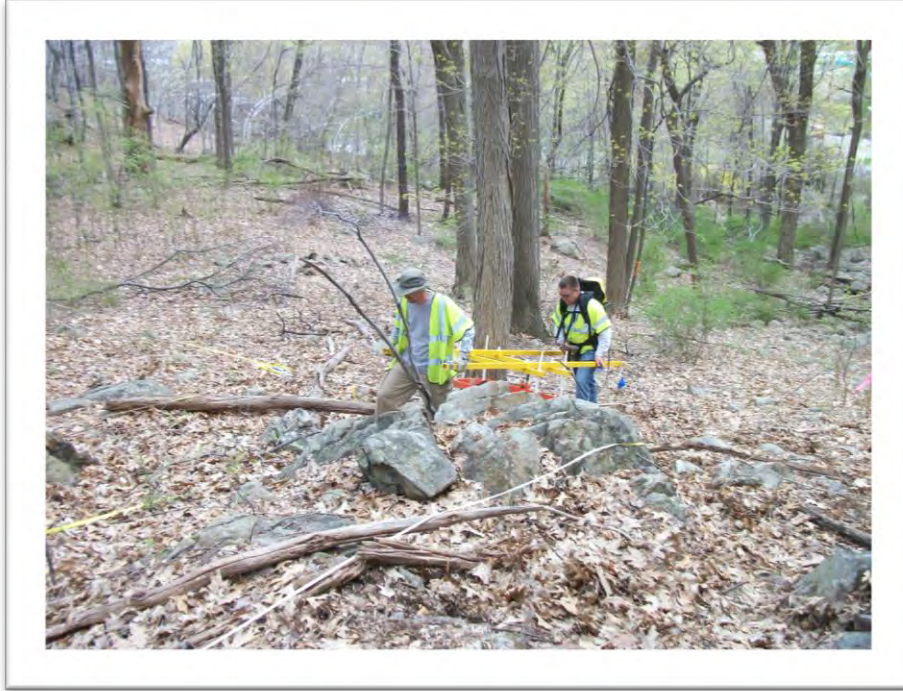
Geophysical Technicians collecting DGM data at grid RD-08 in Redoubt No2 MRS.
