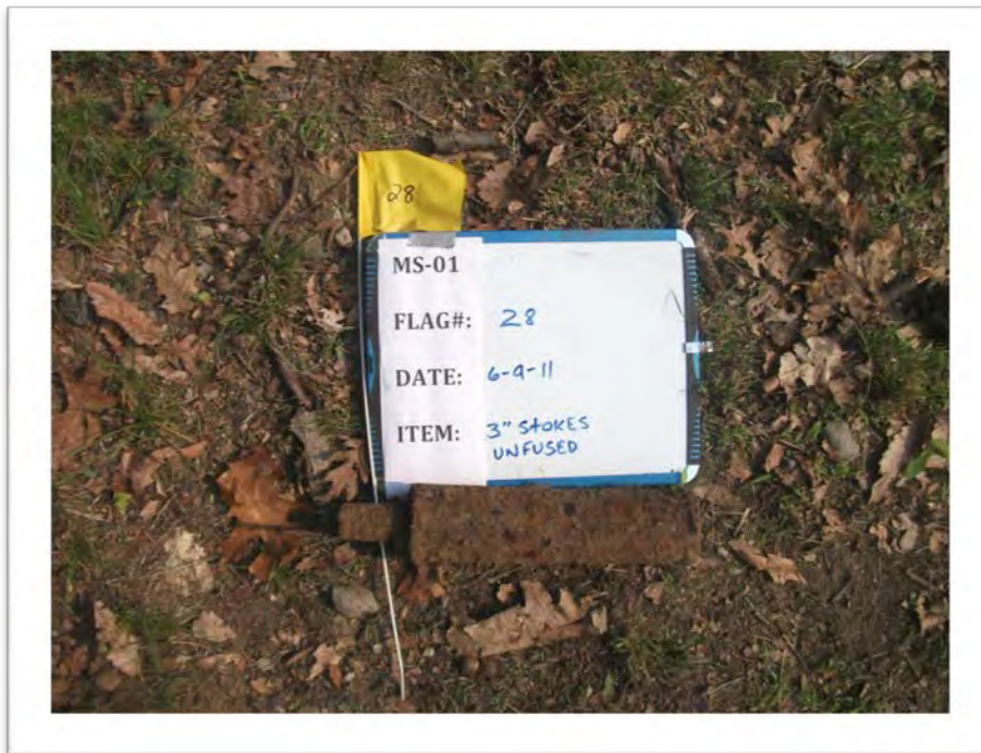
3" Stokes training mortar (unfuzed) recovered from grid MS-01 in Michie Stadium MRS.
