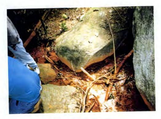
SEEPAGE AT ROCK OUTCROP IN THE MIDDLE OF THE IRON STAINED SLOPE
