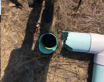
**Photo 4:** View looking downward at damaged GVS-6 at a close up of the broken PVC base.
