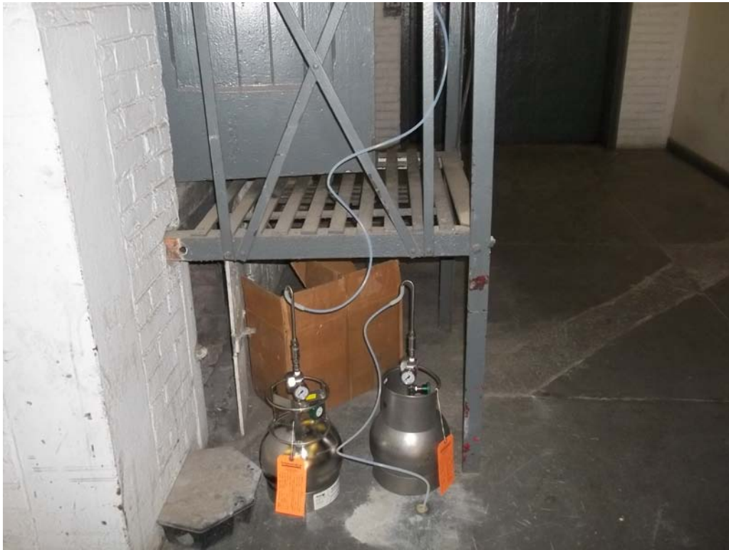
Sub-Slab Sample and Indoor Sample from Breathing Zone, Structure B04
