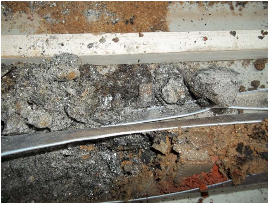
Example of Mica and Fill Identified in Soil Borings
