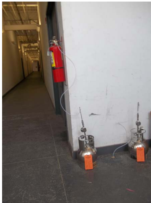
Sub-Slab Sample and Indoor Sample from Breathing Zone, Structure B04
