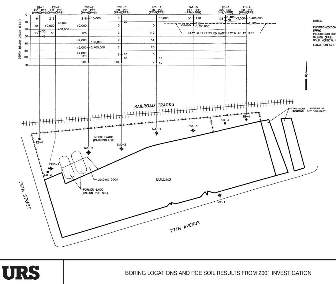
PHOTOIONIZATION DETECTOR (PID) READINGS ARE REPORTED IN PARTS PER MILLION (PPM) PERCHLOROETHYLENE (PCE) LABORATORY RESULTS ARE REPORTED IN PARTS PER BILLION (PPB) BOLD VERTICAL LINE REPRESENTS DEPTH OF BORING LOCATION LOCATION SVE-1 WAS NOT SAMPLED DURING THE INVESTIGATION.
