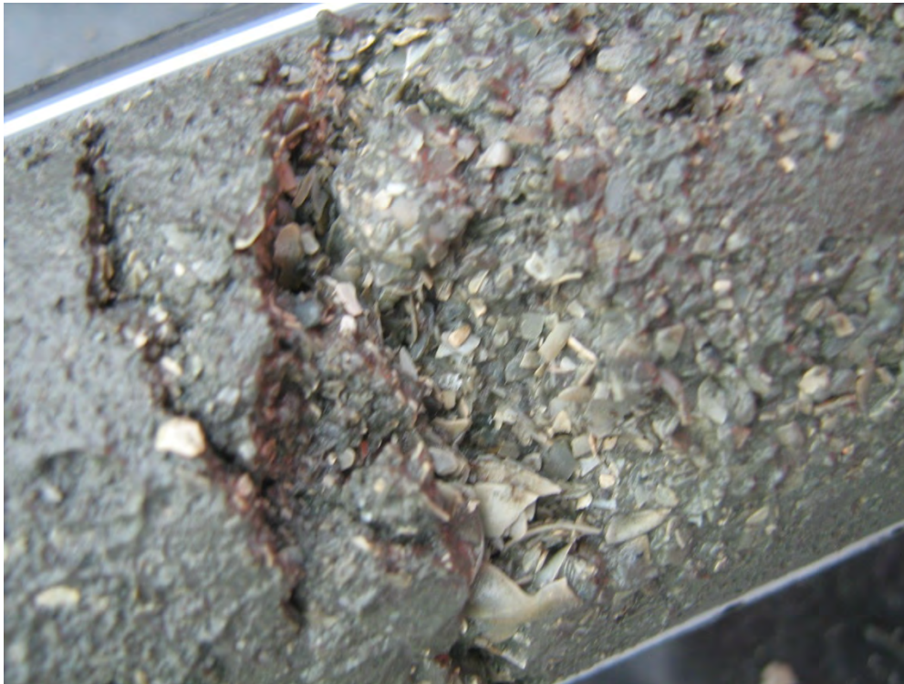
Photo 8: Soil sample from soil boring SB-02 (35 to 40 feet). Note shell fragments.
