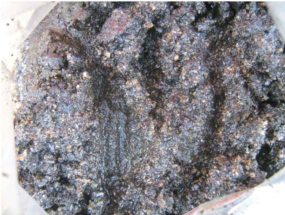
Photo 6: Soil sample from soil boring SB-08 (30 to 35 feet), exhibiting contamination.
