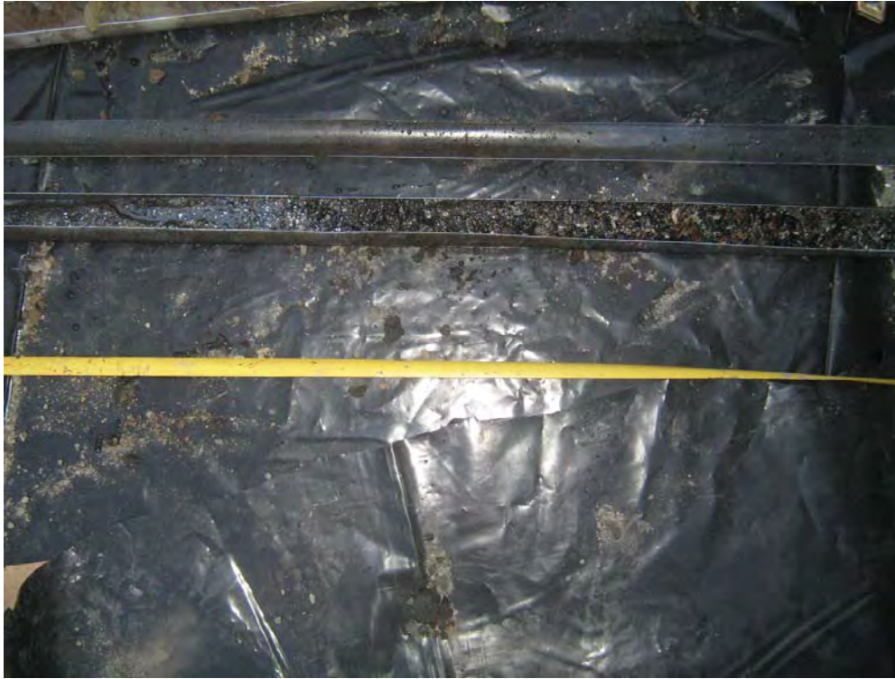
Photo 7: Soil sample from soil boring SB-07 (25 to 30 feet), exhibiting contamination.
