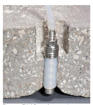
Figure 5. FLX-VP sample connection
