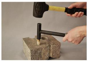
Figure 2. Installing the FLX-VP
