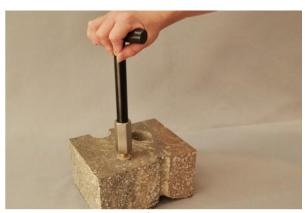
Figure 9. Removing the FLX-VP
