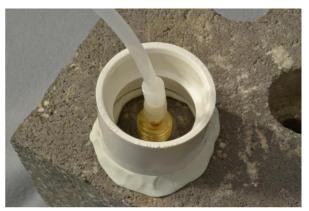
Figure 8. Water dam used for leak detection
