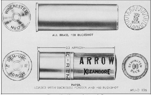
Figure 12. 12 gage shotgun shells
