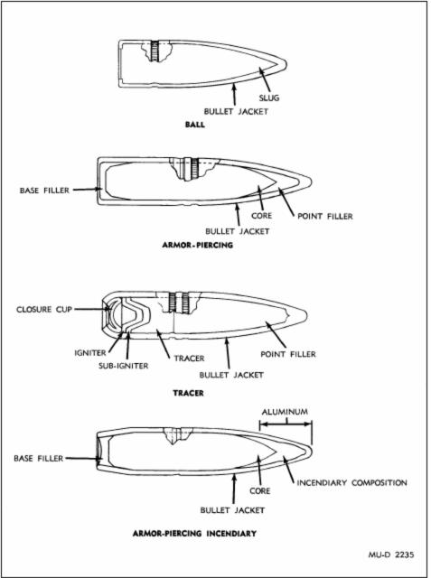
Figure 4. Caliber .30 bullets (sectional)
