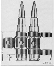
Figure 13. Linked 7.62-mm cartridges
