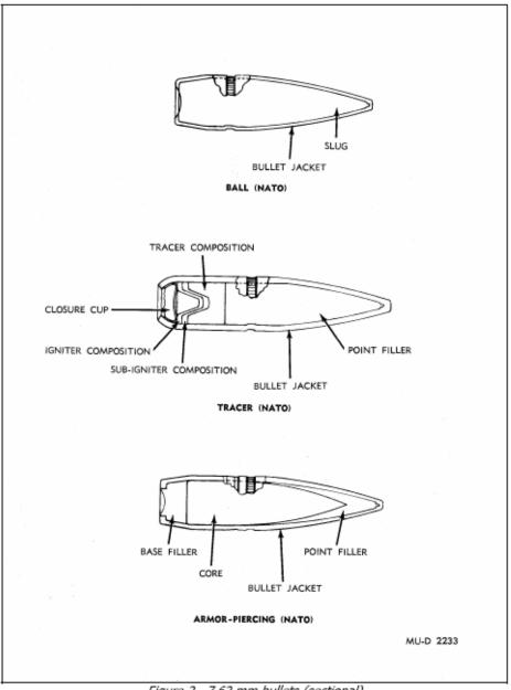
Figure 2. 7.62 mm bullets (sectional)
