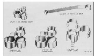
Figure 14. Links for caliber .30 and caliber .50 ammunition
