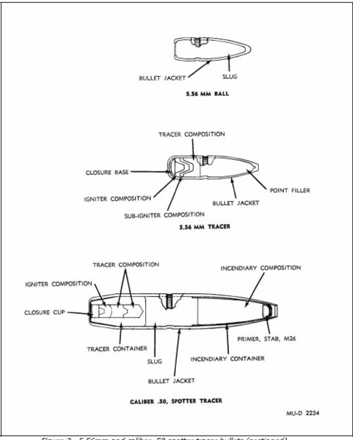
Figure 3. 5.56mm and caliber .50 spotter tracer bullets (sectioned)
