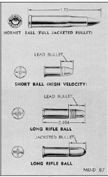
Figure 10. Caliber .22 cartridges
