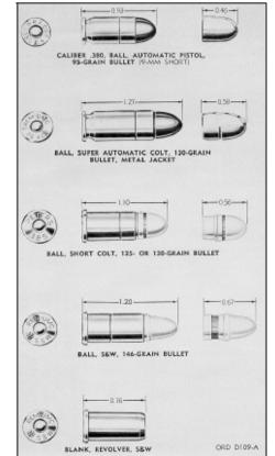
Figure 11. Caliber .38 cartridges
