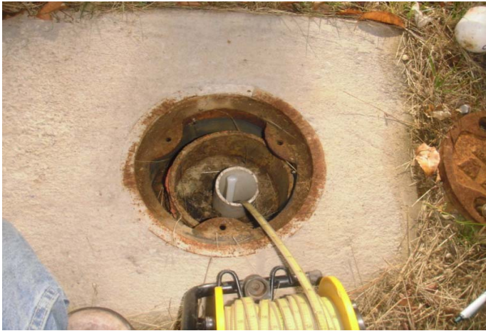
Picture 332- All piezometer wells were gauged with an interface probe to determine water levels.
