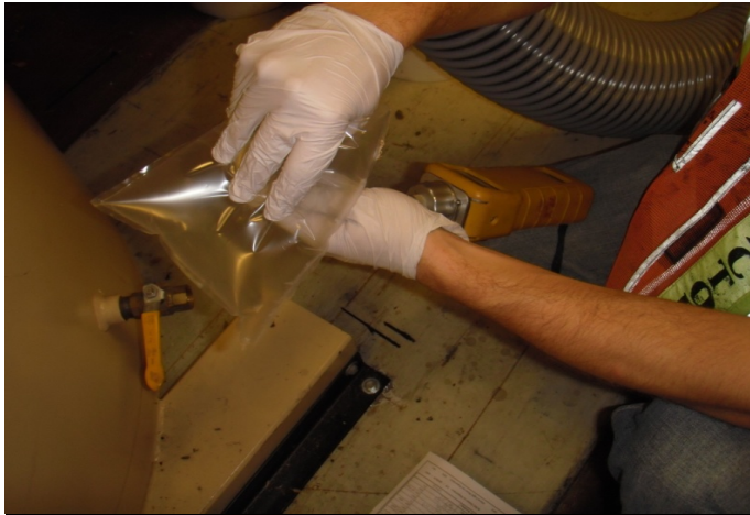
Picture 303- The vapor points within the GAC shed were screened in a Tedlar bag.
