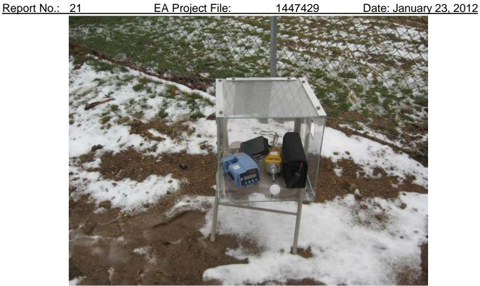
Downwind air monitoring station.
