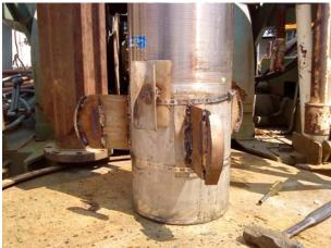
2. Sump to remove water from dumpster
