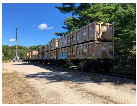
Photograph 7 – Intermodals Loaded on Railcars for Offsite Disposal
