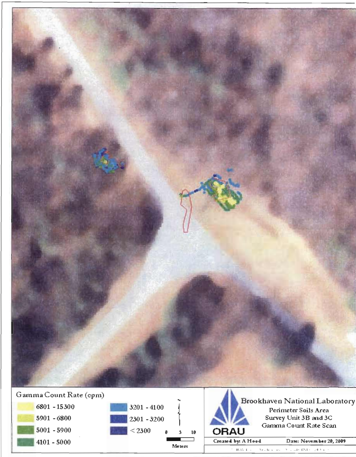
Figure A-5. Perimeter Soils Area Gamma Count Rate Scan Survey Units 3B and 3C
