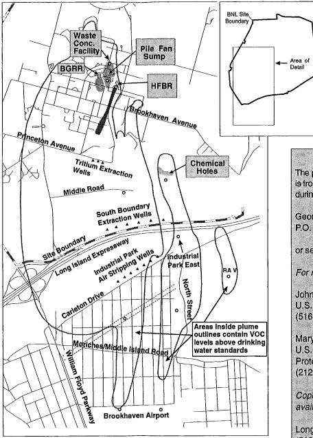
This figure shows the locations of groundwater contaminants at levels above drinking water standards as well as the locations of the tritium and strontium-90 sources. It also indicates proposed locations for treatment systems.
