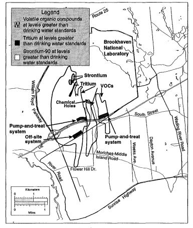
This figure shows the locations of the Operable Unit III groundwater contaminants, and VOC treatment systems. The Chemical Holes are a source of both VOCs and strontium-90.
