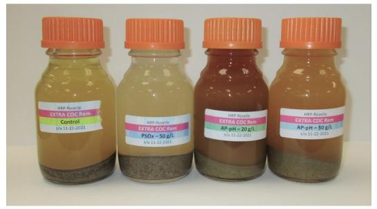
Figure 2. COC Removal Reactors at Day 28 – Follow-up Tests. From left: Control, PersulfOx® 50 g/L, AP-pH-20 g/L, AP-pH-50 g/L.
