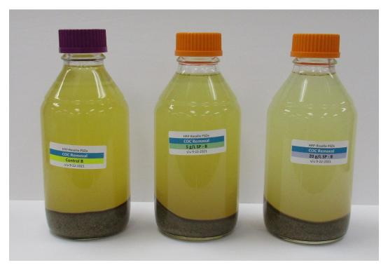
**Figure 1. COC Removal Reactors at Day 28** – *Initial Tests.* From left: Control, PersulfOx® Low, PersulfOx® High.
