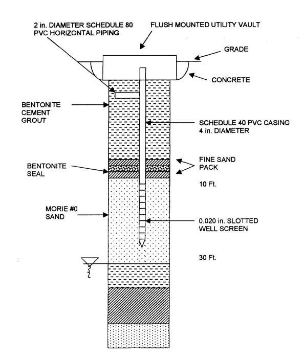
Figure 3 - SVE Well Diagram NOT TO SCALE
