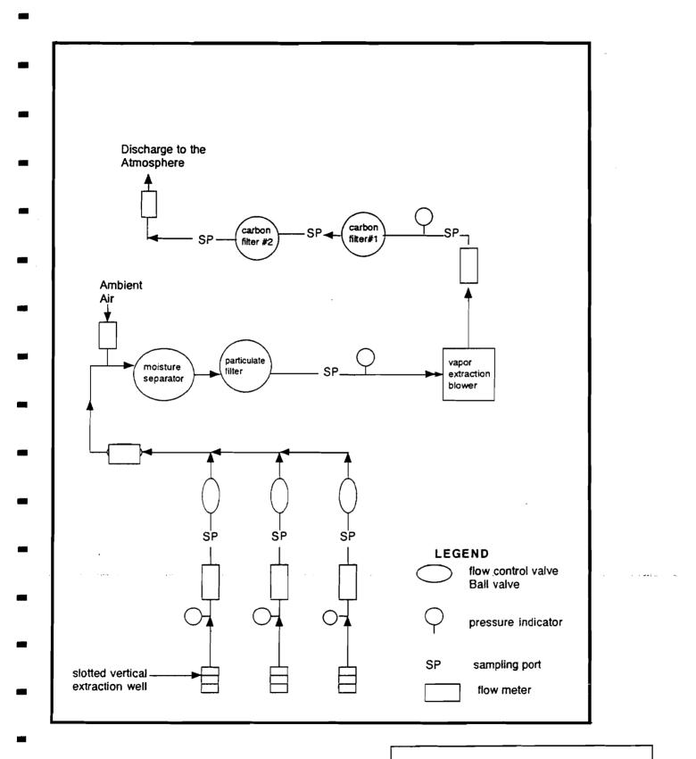
Figure 6 Schmatic Diagram of Soil Vapor Extraction System
