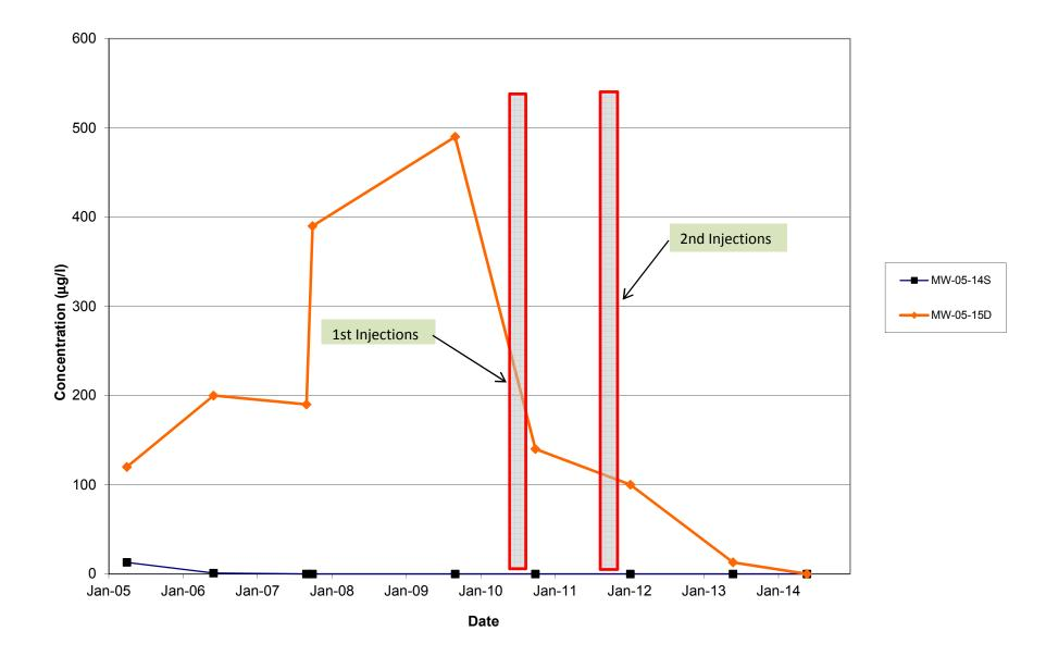
FIGURE 3 CHLOROETHANE CONCENTRATIONS IN WELLS MW-05-14S AND MW-05-15D FORMER COLUMBIA CEMENT COMPANY SITE FREEPORT, NEW YORK
