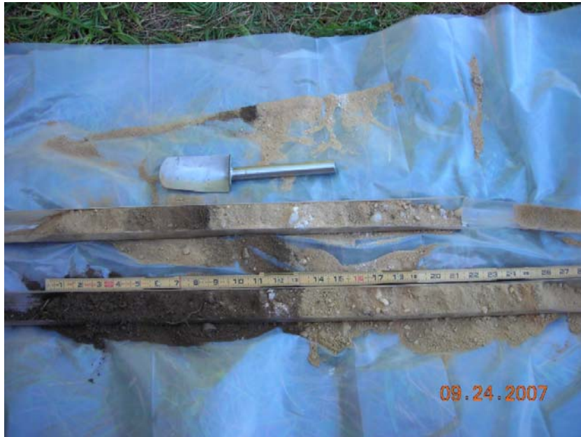
Photo 19 Soil Core from Boring Adjacent to Sampling Location SG-18 Along Northern Property Boundary
