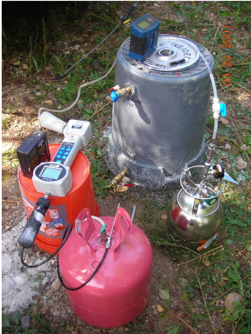
Photo 2 Sampling Location SG-13 Typical Soil Vapor Sampling Set-Up
