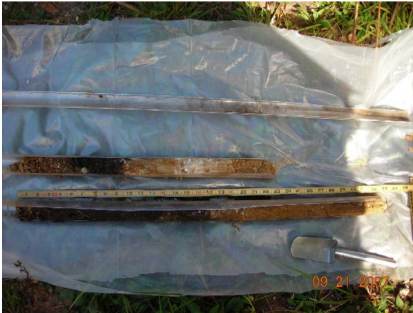
Photo 11 Soil Core from Boring Adjacent to Sampling Location SG-10 Along Southwest Property Boundary
