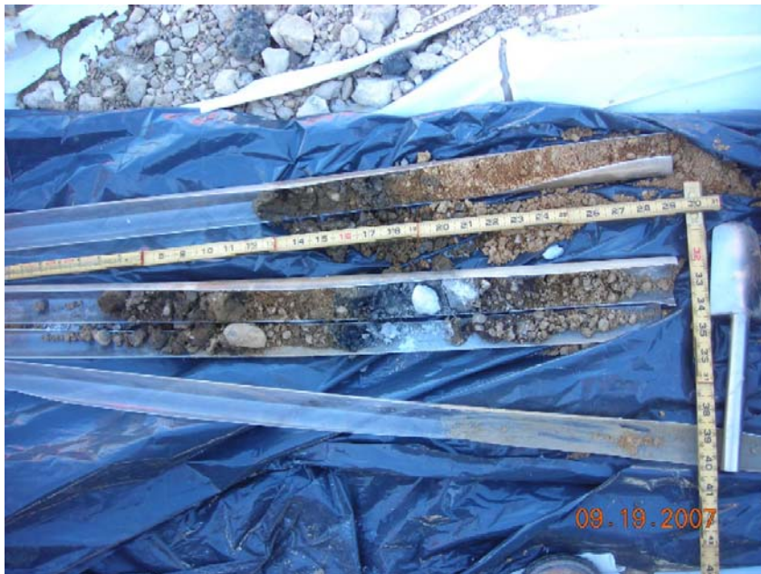
Photo 2 Soil Core from Boring Adjacent to Sampling Location SG-2 Within Former Plant 1 Footprint
