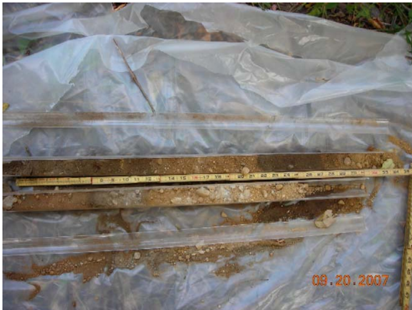
Photo 14 Soil Core from Boring Adjacent to Sampling Location SG-13 South of Former Rainwater Runoff Sump
