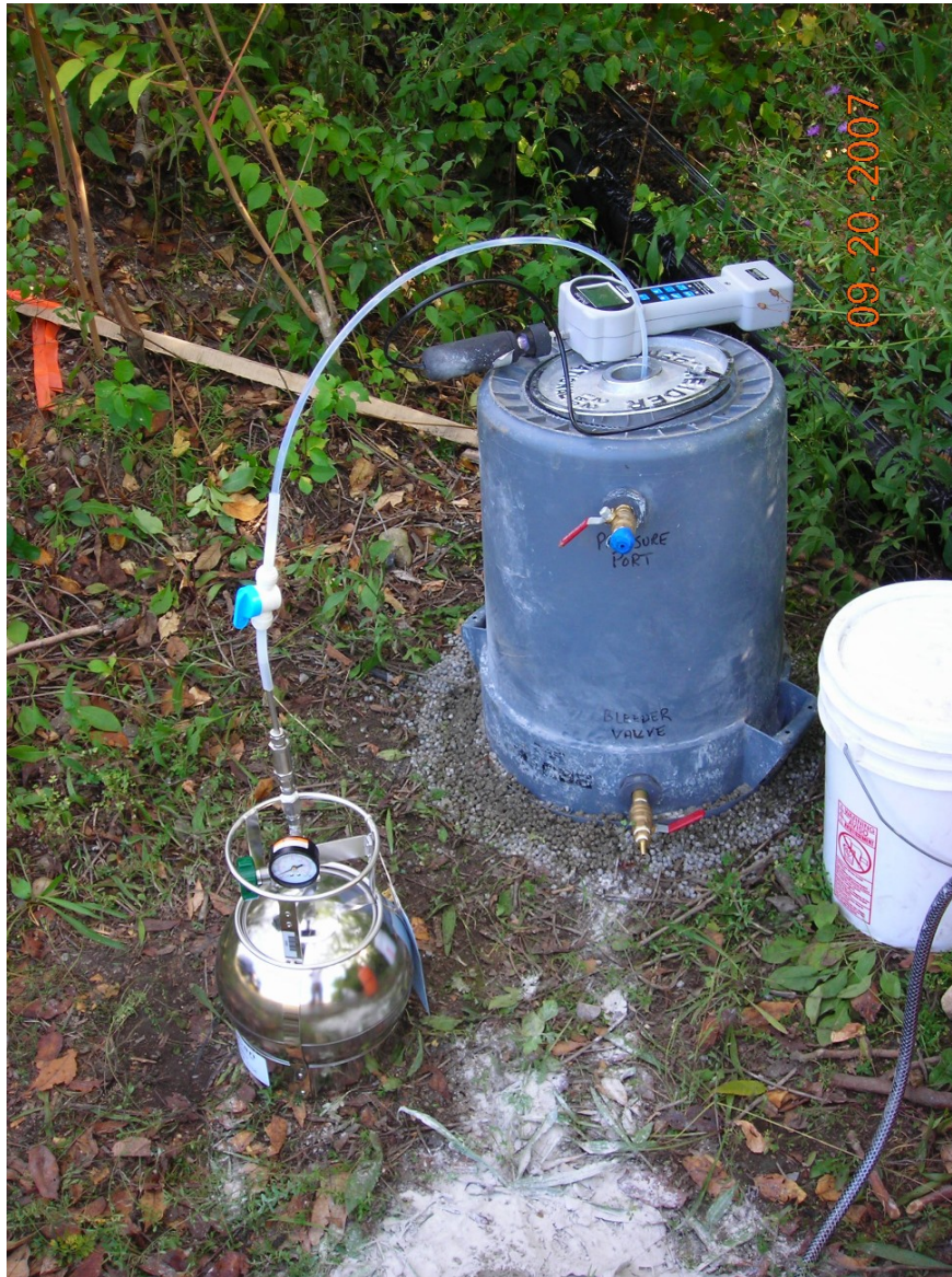
Photo 1 Sampling Location SG-12 Typical Soil Vapor Sampling Set-Up
