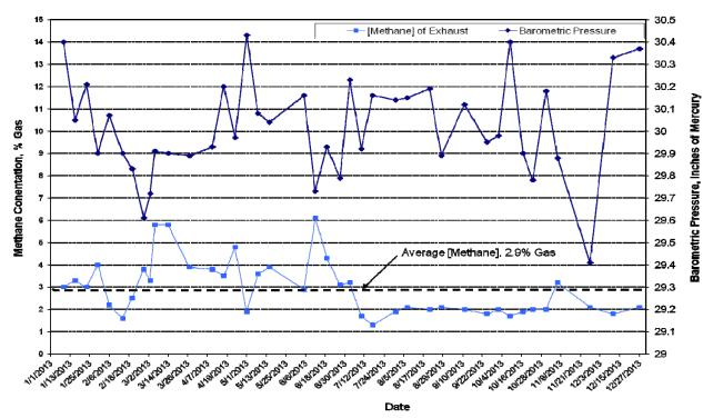
Figure 10. 2013 [Methane] of Landfill Gas Collection System Exhaust
