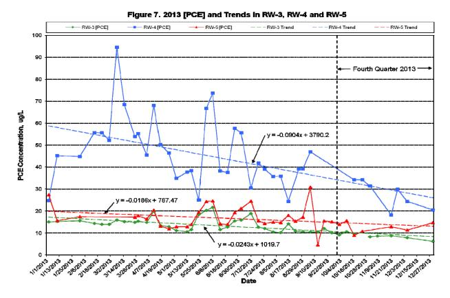
As shown in Figure 7 above, during the fourth quarter of 2013, [PCE] in Recovery Wells RW-3 and RW-4 exhibited decreasing trends, and [PCE] in Recovery Well RW-5 remained relatively constant. [PCE] were highest in Recovery Well RW-4, and lower and similar in Recovery Wells RW-3 and RW-5. Based on the slopes of the trend lines in Figure 7, [PCE] in all three wells exhibited decreasing trends during 2013.
