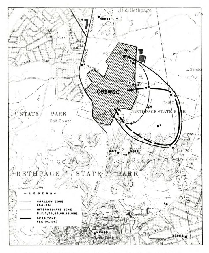
Figure 1-1- APPROXIMATE EXTENT OF LANDFILL LEACHATE PLUME WITHIN 3 HYDROGEOLOGIC ZONES
