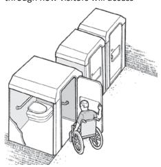
Drawing of an accessible portable toilet with grab bars and a turning space.
